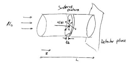
First, the number of scattered photons generated in each incremental thickness is:
