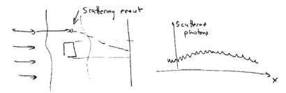
By increasing  $\overline{S}$  and  $\sigma_s$  the scattered photons will reduce both the contrast and the contrast to noise ratio.
