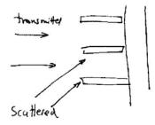
where the gird is made out of some high  $\mu$  material (like Pb, W) that will block any photons that strike it. The grid works principally by cutting down on the acceptance angle for scattered photons,  $\Omega$ :
