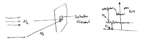
Consider the case where we have  $N_t = N$  transmitted photons and  $N_s$  scattered photons and a signal difference of  $\Delta N$ . The original contrast was:
