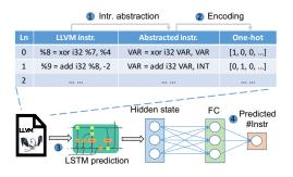
**Figure 6.** The instruction prediction machine learning model. The LSTM recurrently takes in LLVM instruction sequence encodings, and outputs a hidden state which represents the extracted information; The information is then fed into a Fully Connected (FC) layer for regression—i.e., predicting the number of instructions.
