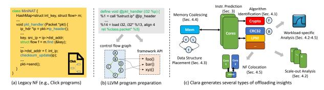
**Figure 2.** The roadmap of Clara and the key techniques. (a) Clara takes in a legacy NF in its unported form (e.g., Click programs). (b) Clara transforms the NF into a low-level Intermediate Representation (IR) using program analysis. (c) Clara uses a combination of program analysis and machine learning techniques to generate several types of offloading insights.
