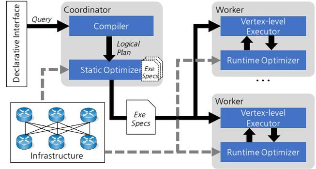
**Figure 3: The GraphRex architecture.** A compiler generates a logical plan from a Datalog query (4.1). The static optimizer then constructs from the logical plan a datacenter-centric execution specification (4.2) that is optimized (5) before the final translation to and evaluation of the physical plan by workers. Grey lines describe dissemination of infrastructure configurations and black lines communication for query execution.
