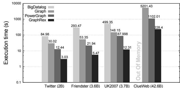
**Figure 1: Performance comparison (log scale) of SSSP between declarative systems: BigDatalog and GraphRex, and low-level graph systems: Giraph and PowerGraph on large graphs. All systems are run in a datacenter with 6 TB RAM and 1.6 K cores in aggregate.**
