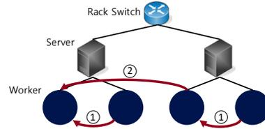
**Figure 12: Hierarchical Global Aggregation in a rack. After worker-level aggregation, intermediate aggregates are shuffled (1) at a server-level, and (2) at a rack-level before finishing global aggregation.**
