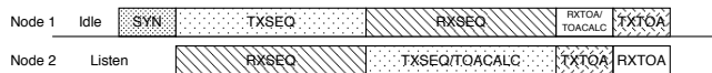
Figure 3: Ranging protocol flow. Exchange is initiated through transmission of a synchronization packet (SYN). The ranging sequence then immediately follows (TXSEQ), with the second node listening (RXSEQ). The nodes then trade roles with the first node listening. Lastly, ToA estimates are traded between nodes to come to a final ToF range estimate (RXTOA/TXTOA).
