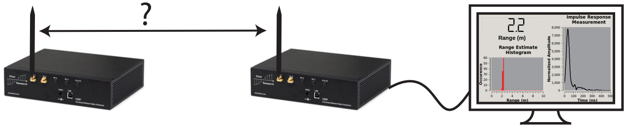
Figure 1: Ranging demo consisting of SR2 implemented on two commodity USRP1 software radios. Range estimates are updated automatically between two autonomous nodes, then sent to a computer for display and visualization of the channel impulse response.
