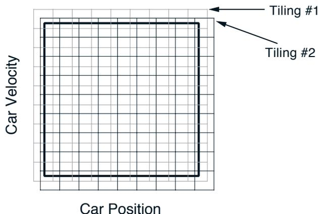
Figure 10. Two  $9 \times 9$  CMAC tilings offset and overlaid over the continuous, two-dimensional state space of the Mountain-Car task. Any state is in exactly one tile/box/feature of each tiling. The experiments used 5 tilings, each offset by a random fraction of a tile width.
