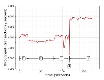
Fig. 7: Throughput of MySQL read\_only before, during, and after code replacement. 95% tail latency degrades from 1.00ms to at most 1.55ms during code replacement.
