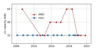
Fig. 1: AMD & Intel per-core L1i capacity over time
