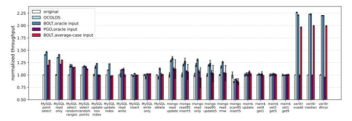
Fig. 5: Performance of OCOLOS (light blue bars) compared to BOLT using an oracle profile of the input being run (dark blue bars), Clang PGO using the same oracle profile (purple bars) and BOLT using an average-case profiling input aggregated from all inputs (pink bars). All bars are normalized to original non-PGO binaries (white bars).
