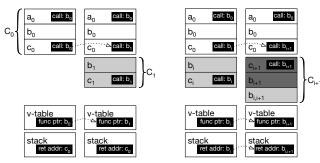
Figure 4b: Starting state of the address space (left) and state after code replacement (right)
