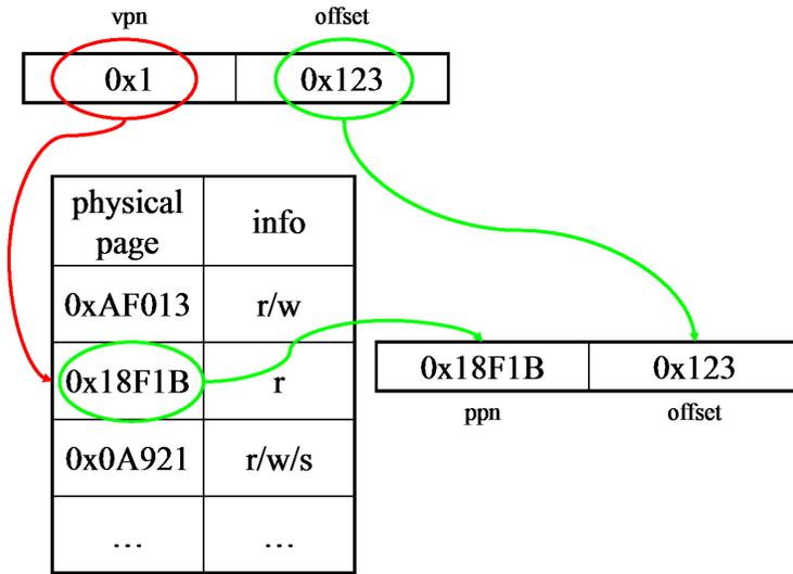
Figure 1: Translation procedure in paging for a 32-bit address space with 4KB pages.
