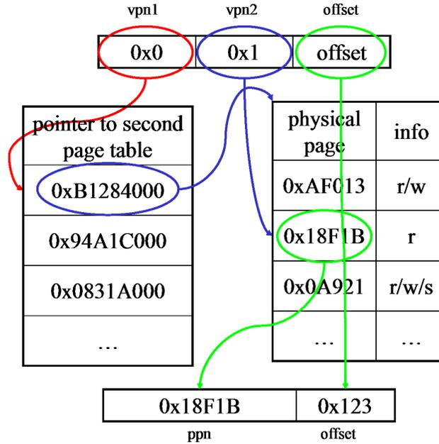
Figure 2: Translation procedure in multilevel paging for a 32-bit address space with 4KB pages
