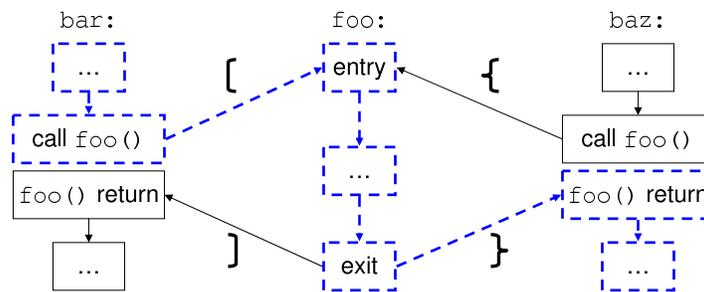
Fig. 6: Interprocedural control flow graph for two calls to the same function. The dashed path is infeasible, since  $foo()$  returns to a different context than the one from which it was called. The infeasible path corresponds to the unbalanced string “[}”.
