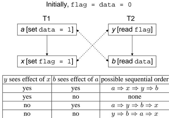
Fig. 1: A program fragment consisting of four memory accesses in two threads. The solid edges correspond to order in the execution stream of each thread, and the dashed edges are conflicts. Of the four possible results of thread 1 visible to thread 2, the second is illegal since it does not correspond to an overall execution sequence in which operations are not reordered within a thread.
