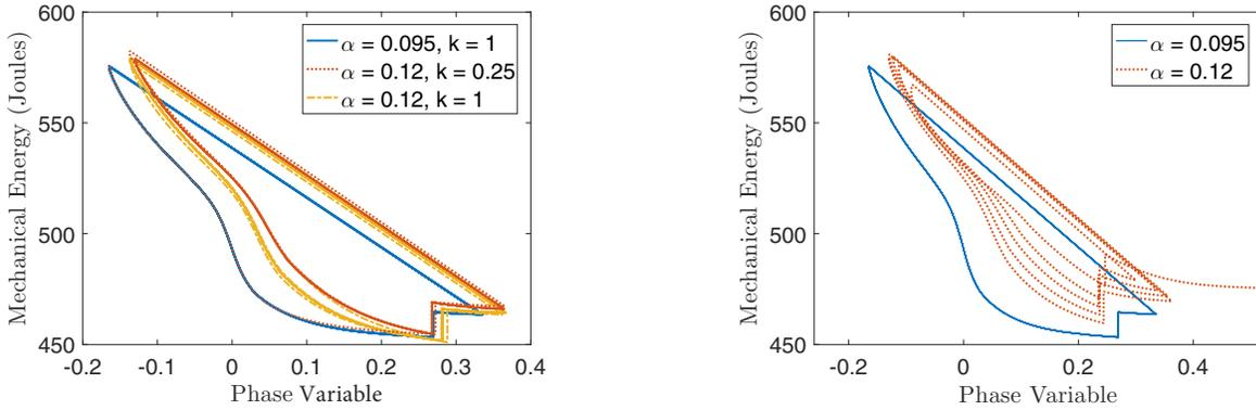
Fig. 5: Biped limit cycle with slope  $\alpha = 0.12$  rad compared with the nominal slope  $\alpha = 0.095$  rad. The left figure shows the change in biped's phase portrait when varying slope and gain using the PBC. The right figure shows the biped's phase portrait without the PBC.
