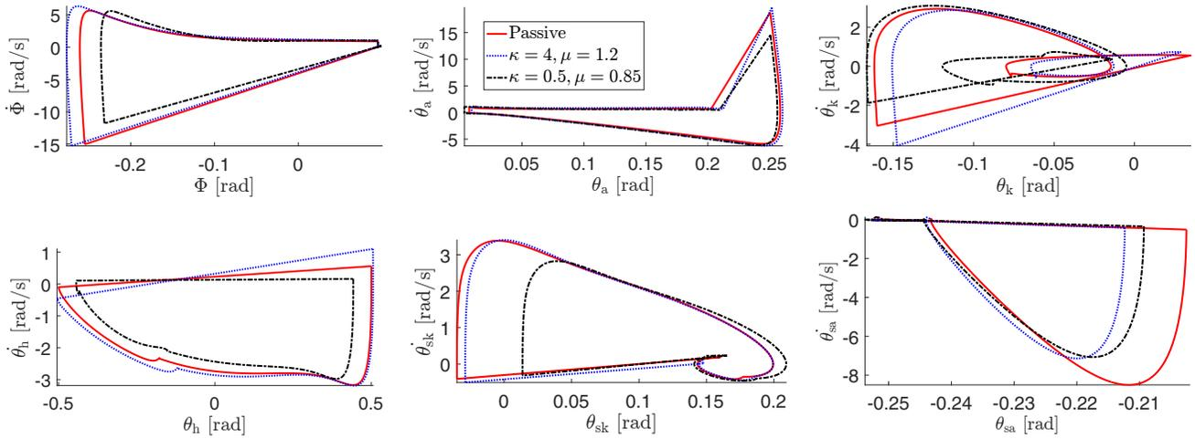
Fig. 4. Phase portraits of  $\phi$  (top left), stance ankle (top center), stance knee (top right), hip (bottom left), swing knee (bottom center), and swing ankle (bottom right) of the passive gait and the controlled gaits ( $\kappa = 4, \mu = 1.2$  and  $\kappa = 0.5, \mu = 0.85$ ) during one steady step. All these figures share the same legend.
