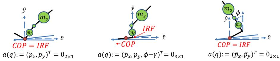
Fig. 2. Heel contact condition (left), flat foot condition (center), and toe contact condition (right) during single-support period on a slope with angle  $\gamma$ . The position of the heel is given by  $(p_x, p_y)$  and the position of the toe is given by  $(\bar{p}_x, \bar{p}_y)$ .
