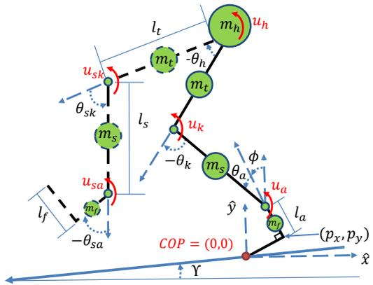
Fig. 1. Kinematic model of the biped, where the stance leg is shown in solid black and the swing leg in dashed black. For simulation study, we assume the biped is walking on a slope with angle  $\gamma$ . The red arcs indicate the joints that are actuated by both the exoskeleton and human, and COP denotes the Center of Pressure.
