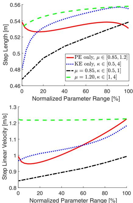
Fig. 3. The step length and step linear velocity with four different shaping strategies during Lyapunov funneling process. The two figures share the same legend and are plotted with normalized  $x$ -axes, e.g.,  $\mu = 0.85$  indicates 0% and  $\mu = 1.2$  indicates 100% on the  $x$ -axes in the PE curves.
