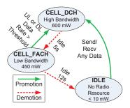
Figure 1: RRC State Machine of a large UMTS carrier in the U.S. The radio power consumption was measured by a Monsoon power monitor [3] on a Google Nexus One (HTC Passion) smartphone. More details can be found in [17].
