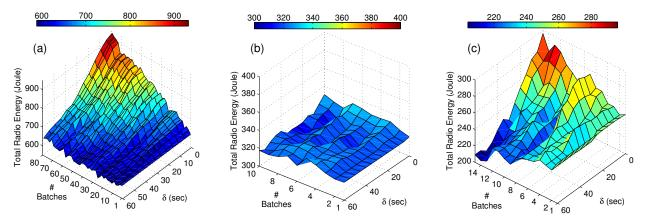
Figure 19: Jointly applying piggyback (varying  $\delta$ ), batching (varying the number of batches), and fast dormancy (the timer is 5s) on target transfers for the three apps: (a) Pandora (b) Dict (c) News. Piggyback and batching can be (a) compatible, (b) ineffective, or (c) incompatible.
