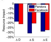
Figure 16: Resource savings of jointly using fast dormancy (the timer is 5s) for periodic transfers, piggyback ( $\delta$ =30s), and batching (increasing the periodicity to 3 minutes).
