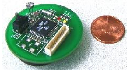
Figure 8: A TinyOS-based Mote: This “mote” includes a 4MHz microcontroller, a software-driven radio, and an application that coordinates with neighboring motes to discover an ad-hoc sensor network routing topology.
