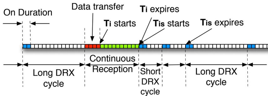
Figure 2.3: Illustration of the LTE DRX in **RRC\_CONNECTED**.
