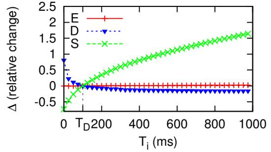
Figure 6.9: Impact of the LTE tail timer  $T_{tail}$ . Figure 6.10: Impact of DRX inactivity timer  $T_i$ .
