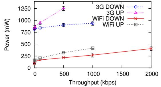
Figure 6.4: Power-throughput curve for 3G and WiFi.
