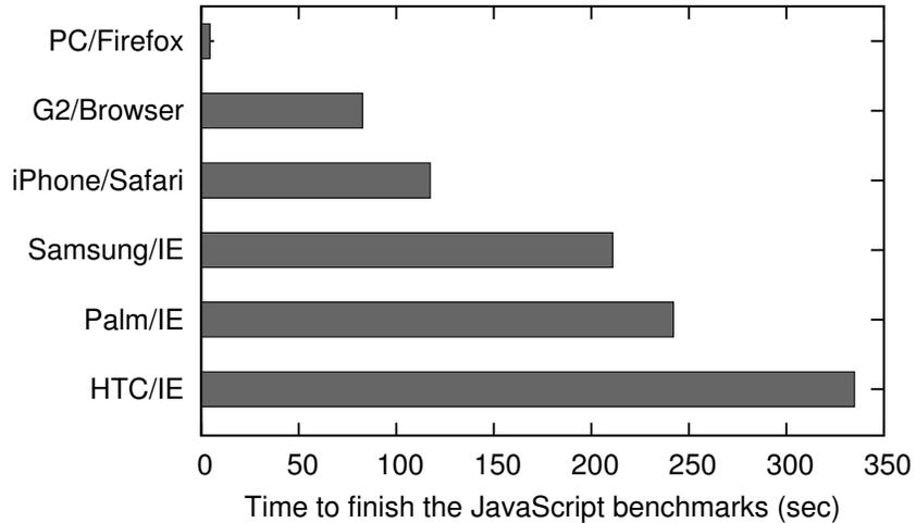
Figure 4.3: Script execution speed for different platforms in 2009.
