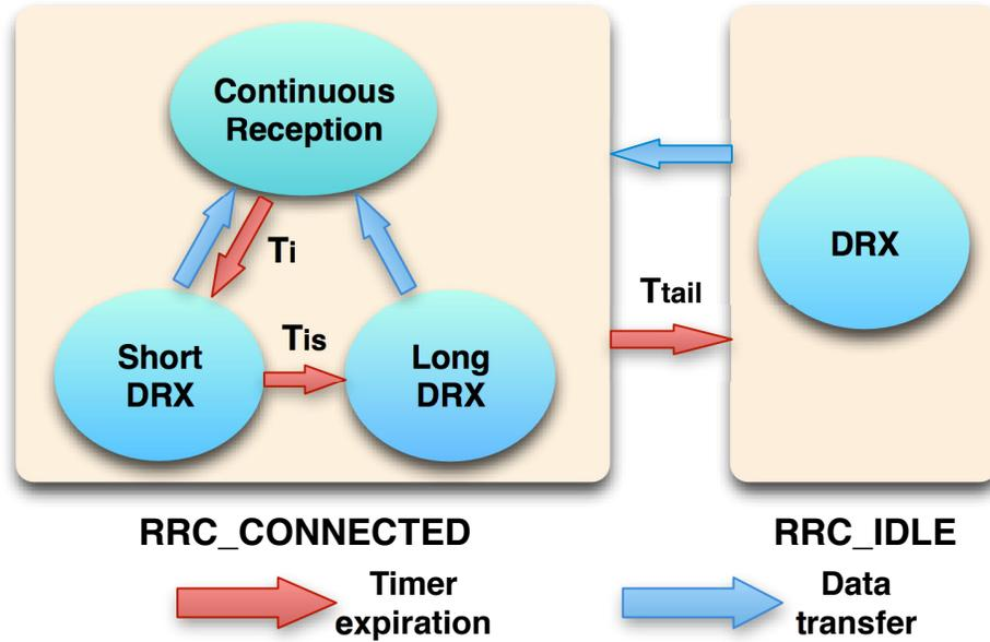
Figure 2.2: RRC state transitions in LTE network.
