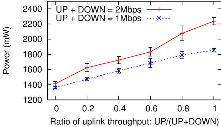
Figure 6.5: Power of simultaneous uplink and downlink transfers.
