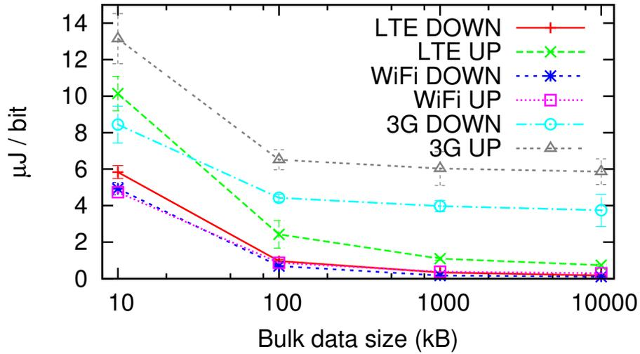
Figure 6.6: Energy per bit for bulk data transfers.
