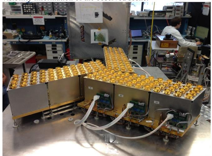
**Figure 1.** The GeoSTAR-III instrument comprising 144 receivers operating at 180 GHz with a CMOS-based correlator subsystem.
