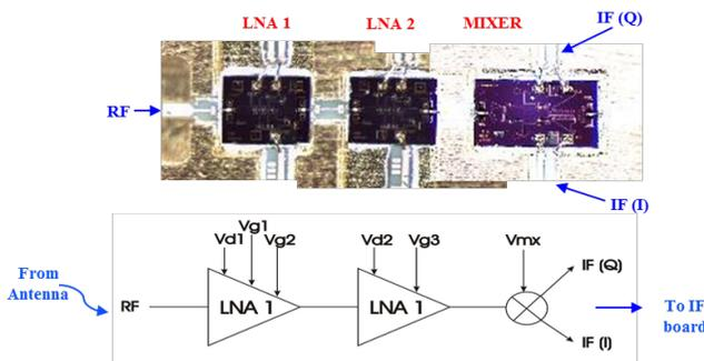
**Figure 2** Block diagram of the MIMRAM module and photo of the assembly. Two low noise amplifier MMICs provide low noise and high gain, and the second harmonic I-Q mixer MMIC enables quadrature conversion to baseband with low LO power.
