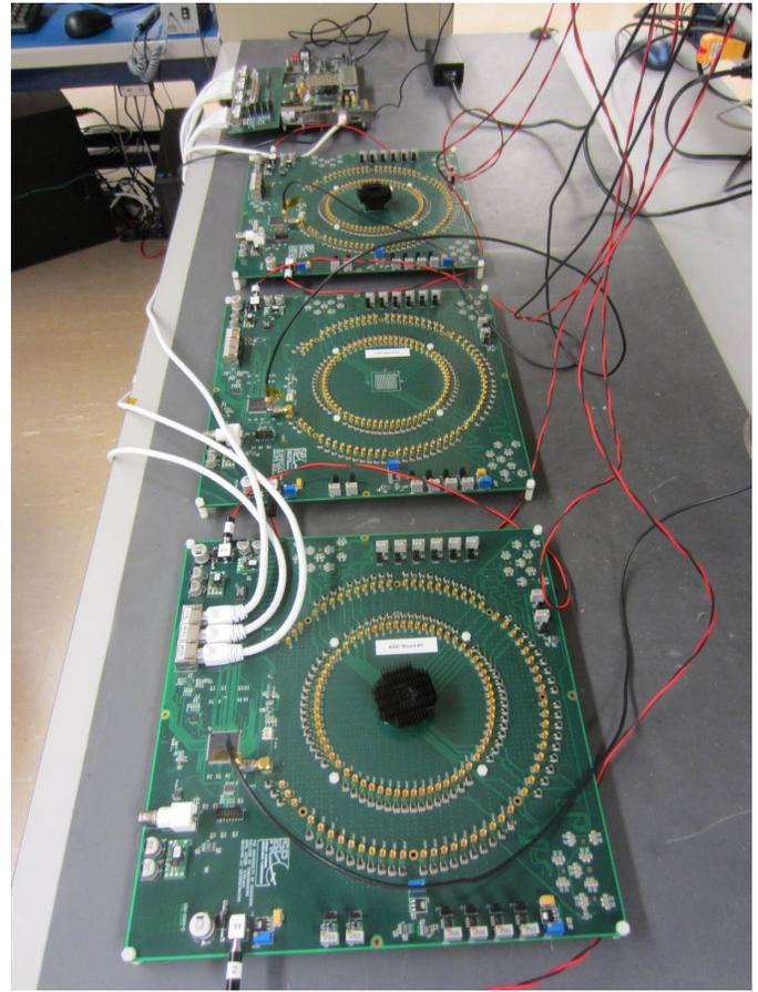
**Figure 4.** The correlation subsystem comprising 3 ASIC on boards and an FPGA-based readout circuit.
