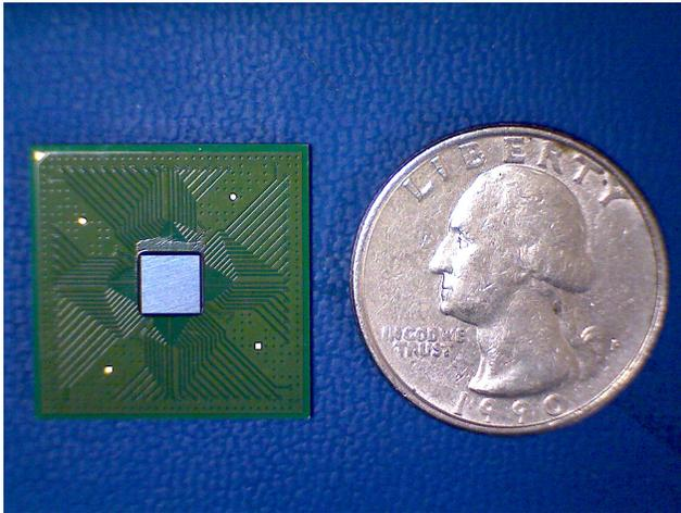
**Figure 3** Packaged 64x64 A/D Correlator ASIC chip.
