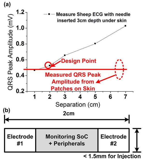
Fig. 2. (a) Measured QRS peak amplitude versus electrode (use needles as the electrodes directly) separation under the skin in a sheep experiment. Note that with  $> 2$  cm separation, the amplitude is larger than the traditional approach with two patches attached to neck and wrist. (b) Dimensions of the proposed system.
