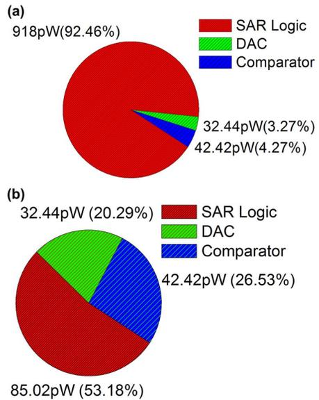
Fig. 9. (a) SAR ADC power breakdown with ADC logic implemented using HVT standard cells. Note that SAR logic consumes 92% of total power when operating at 500 Hz. (b) SAR ADC power breakdown with custom asynchronous logic.
