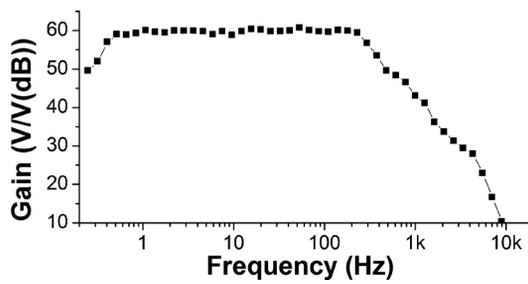
Fig. 18. Measured frequency response of the amplifier with the midband gain set to 59 dB.
