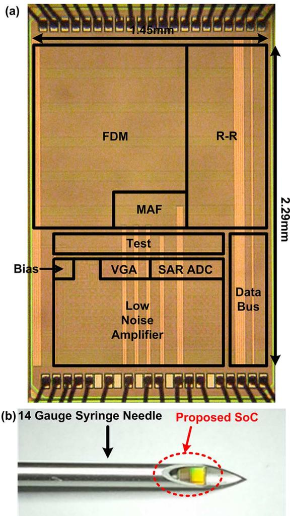
Fig. 17. (a) Die photograph of proposed SoC in 65 nm LP CMOS. (b) Photograph of proposed SoC and a 14 gauge syringe needle.
