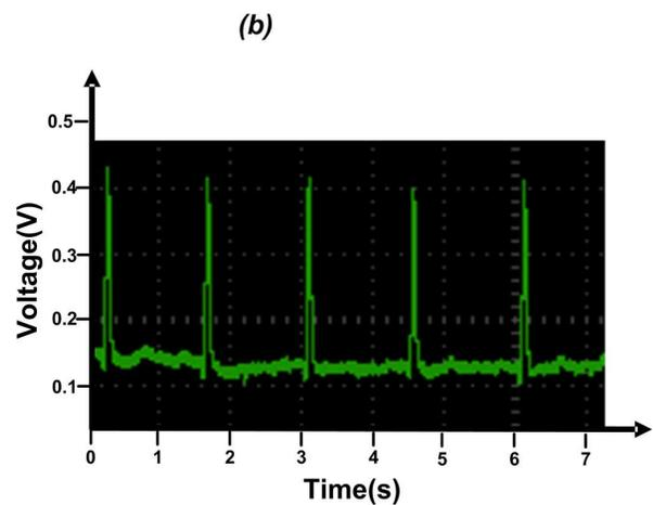
Fig. 20. (a) Test setup of the Human Chest Experiment. (b) Amplified waveform observed from the amplifier output terminal by the Agilent oscilloscope. The Vol/Div is 100 mV/Div and the Time/Div is 0.5 s/Div.
