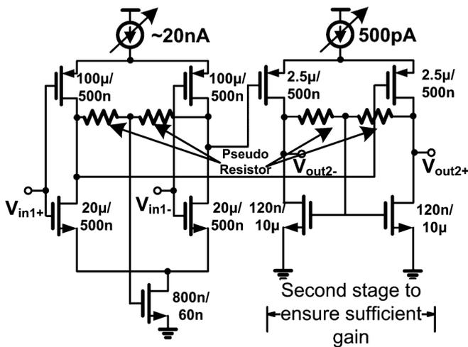
Fig. 7. Core amplifier inside the CCIA.
