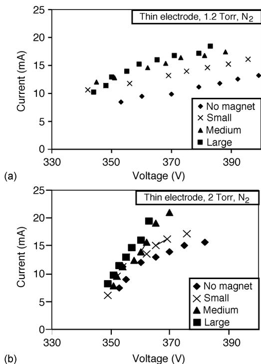
Fig. 6. Measured plasma current as a function of dc voltage at (a) 1.2 and (b) 2 torr.
