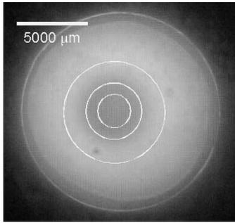
Fig. 4. Local confinement of air microplasma, at 1.2 torr using large magnet. Rings denote magnet profile.
