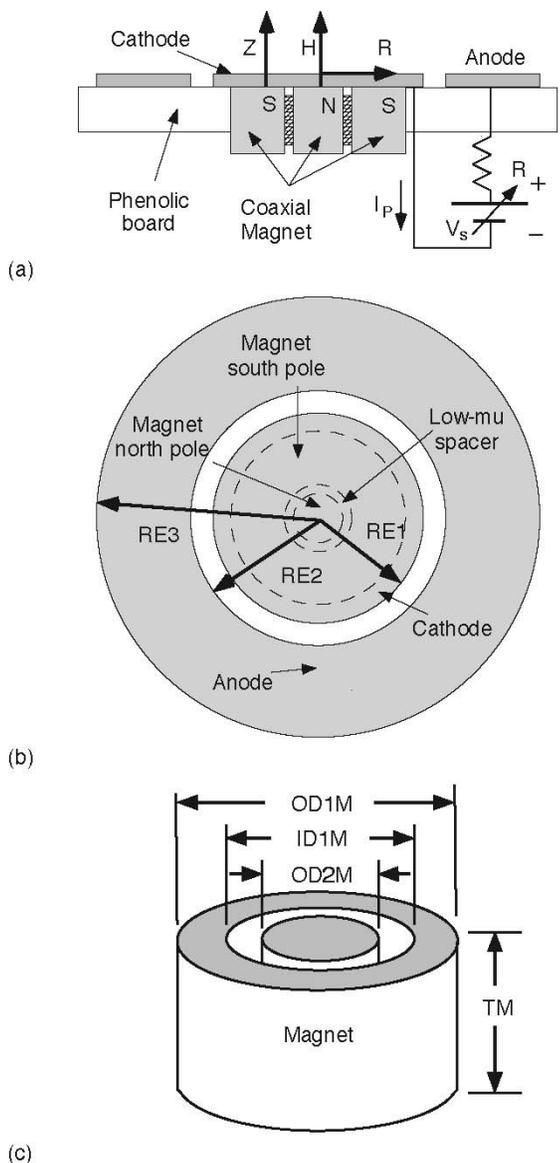
Fig. 1. Schematic illustrating the miniaturized magnetron. (a) Cross section of complete setup showing coordinate system. (b) Top view. (c) Magnet configuration.
