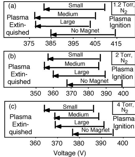
Fig. 5. Plasma ignition and plasma termination with the various magnet sizes for (a) 1.2; (b) 2; and (c) 4 torr.
