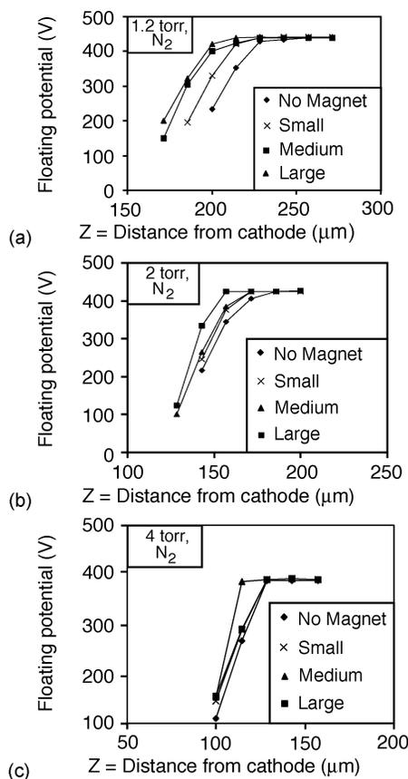
Fig. 8. Floating potential used to measure sheath dimensions: (a) 1.2; (b) 2; and (c) 4 torr.
