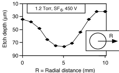
Fig. 10. Etch depth in silicon radially along the ring for a 55-min etch at 1.2 torr with SF<sub>6</sub> gas. Microplasma was operated at 450 V, 0.46 A.
