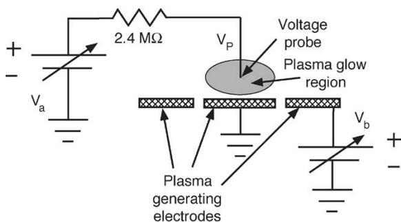
Fig. 7. Circuitry used to measure plasma floating potential.
