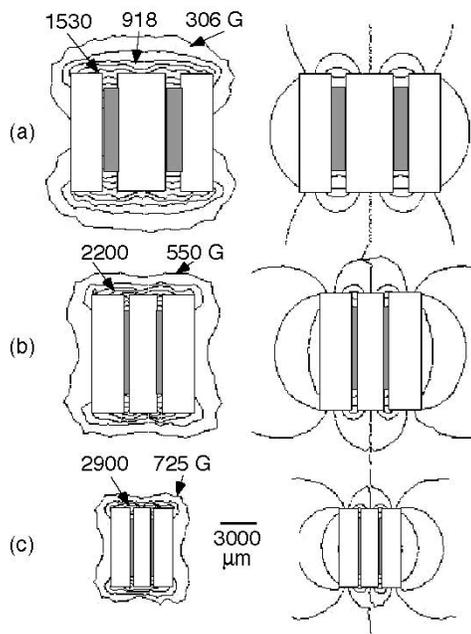
Fig. 2. Simulations of magnetic (left) equipotential surfaces and (right) field lines for (a) large; (b) medium; and (c) small magnet.
