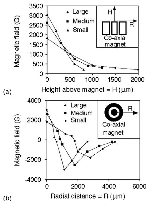
Fig. 3. Measured magnetic field distance  $H$  above magnet (a), and in radial direction (b) for coaxial magnets.
