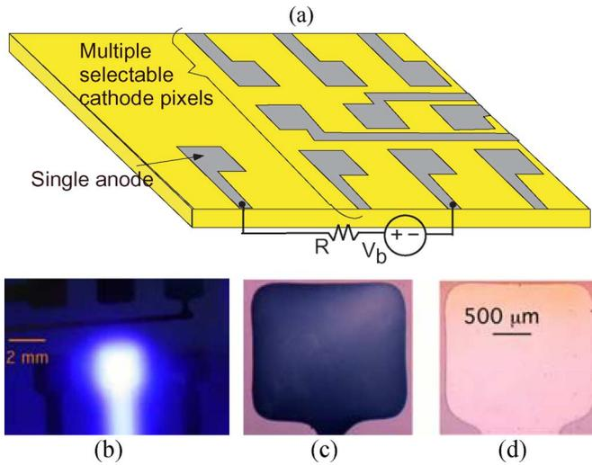
Fig. 1. Microplasmas can be independently generated on electrodes patterned on the wafer substrate. (a) Single anode serving multiple cathode pixels. (b) Localized glow on a cathode pixel at 2 torr and 430 V, in  $N_2$ . (c) Powered cathode pixel in an array after 5 min of deposition at 1.2 torr and 300 °C. (d) Unpowered cathode pixel from the same array showing no deposition.
