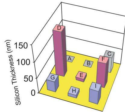
Fig. 2. Maximum silicon thickness per pixel on the array of Fig. 1(a).
