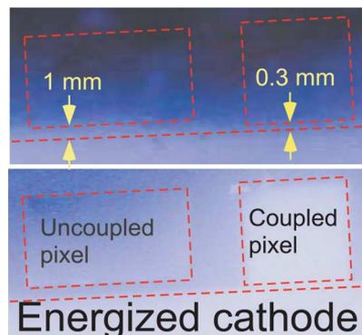
Fig. 5. Floating electrodes proximate to a cathode in N<sub>2</sub> microplasma at 4 torr (above) and 2 torr (below), demonstrating how pixels close to the cathode can be selectively targeted for deposition.
