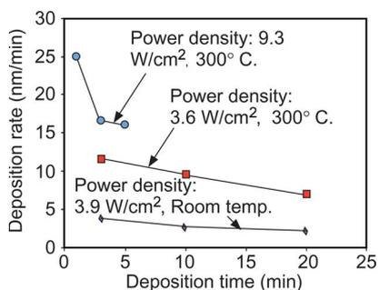
Fig. 3. Silicon deposition rates versus time for varying power densities and temperatures at 1.7 torr and 100/100 sccm silane/argon gas flow.
