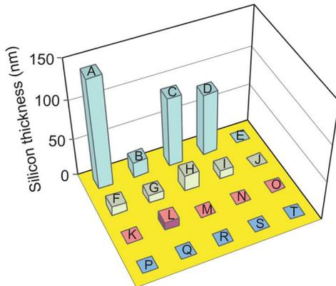
Fig. 7. Silicon thickness per pixel on floating array. Pixel coupling is greatest at 1.4 torr. Deposition rate is highest at 2.1 torr. All depositions were performed at room temperature.
