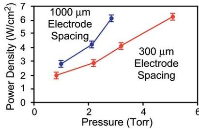
Fig. 6. Power densities and pressures that allow plasma coupling for two different spacings between a powered and a floating electrode. Higher power densities are required for plasma coupling as electrode spacing is increased and as ambient pressure is increased.
