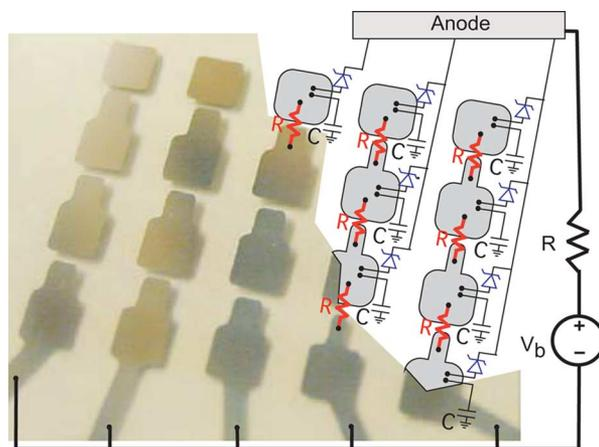
Fig. 4. Microplasmas couple to proximate floating electrodes in an array. The level of coupling is determined by electrode spacing, operating power, and pressure. The equivalent electrical circuit due to the plasma is shown in the cutout.
