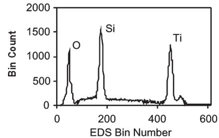
Fig. 8. EDS elemental analysis of pixel G in Fig. 7, detecting Ti (electrode material), Si, and O.
