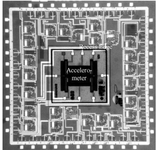
**Figure 2.** An optical micrograph of a capacitive polysilicon microaccelerometer in a recess, surrounded by CMOS sense circuitry.
