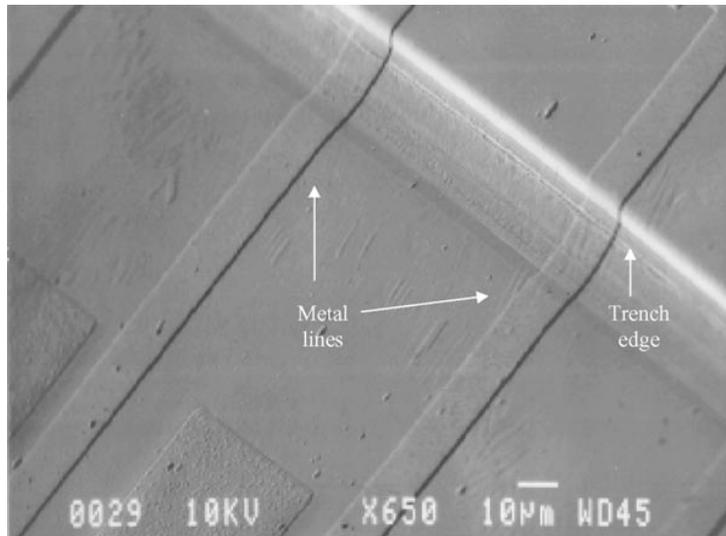
**Figure 3.** A scanning electron micrograph of the aluminum lead transfer over sidewalls of the recess.
