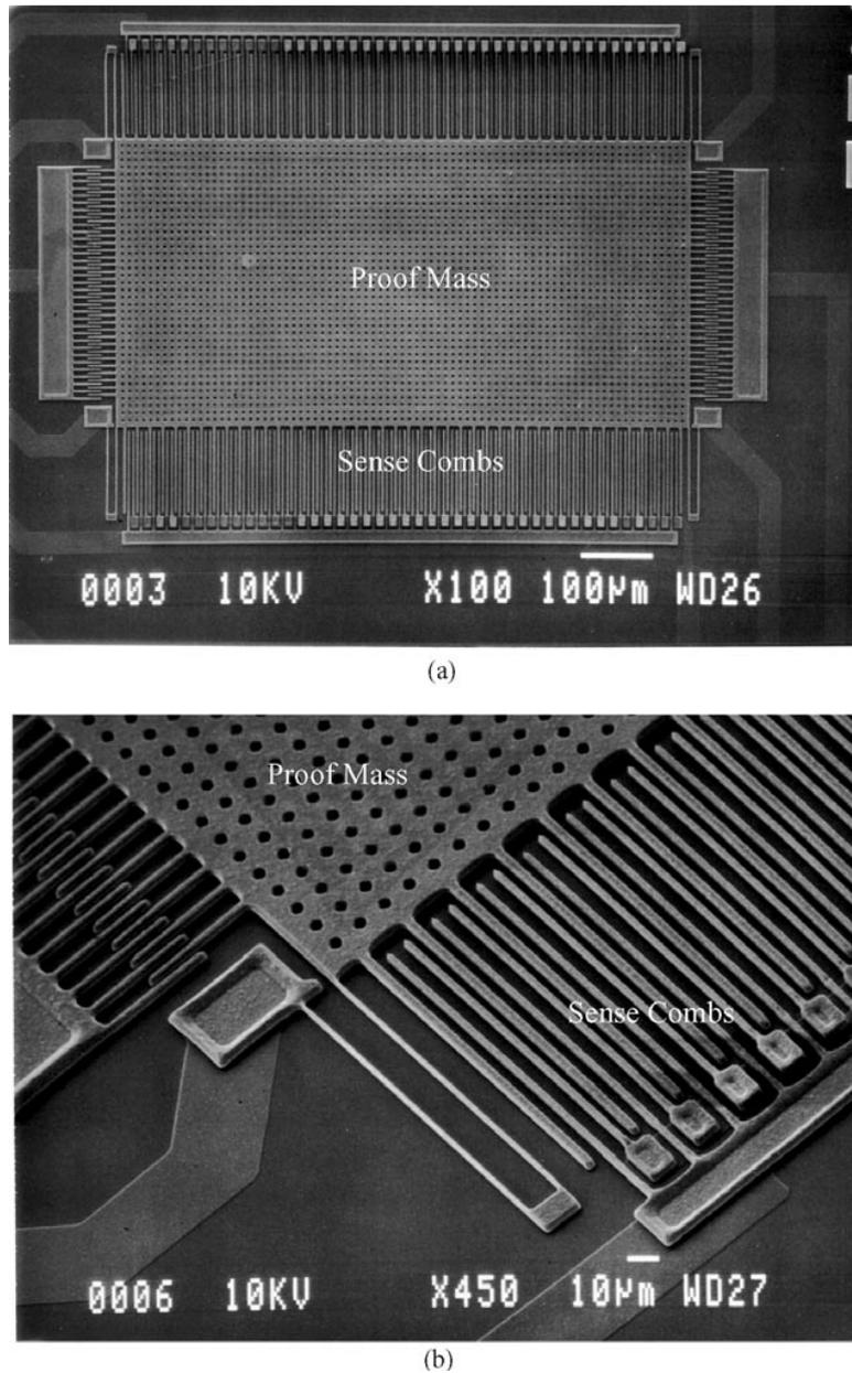
**Figure 4.** (a) A scanning electron micrograph of a capacitive microaccelerometer; (b) a close-up of one corner, showing the sense electrodes.
