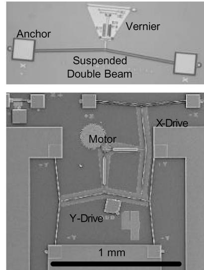
Fig. 2. Fabricated polysilicon microactuators: (a-upper) Optical micrograph of a T4 device, (b-lower) SEM image of a rotary micromotor that used such actuators.
