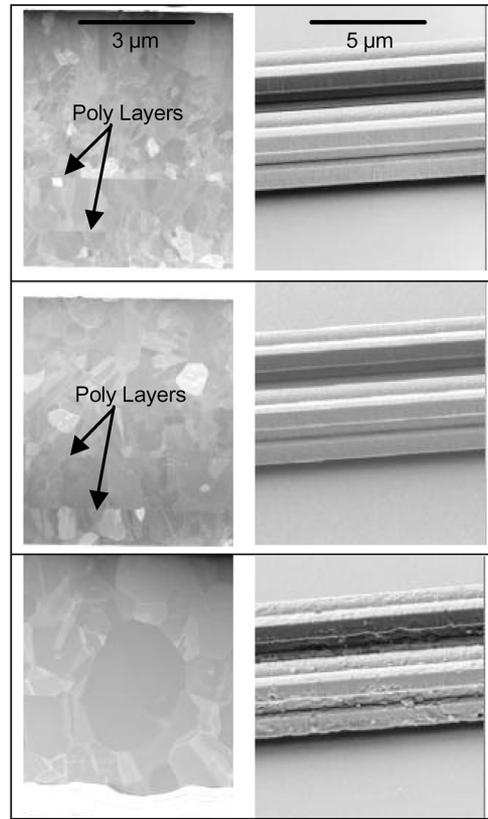
Fig. 11. TEM (left column) and SEM (right column) of bent-beams subjected to different levels of actuation power: (a-top) an unheated section of bent-beam, (b-middle) 58 million cycles at 24 mW, and (c-bottom) 30 million cycles at 43 mW.
