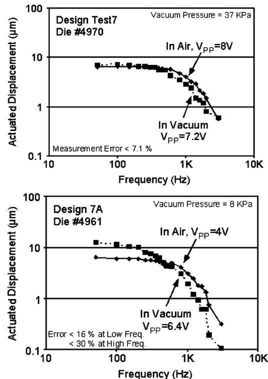
Fig. 4. Measured polysilicon actuator bandwidth (a-upper) for single and (b-lower) cascaded beam designs.
