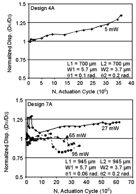
Fig. 9. Displacement variation for polysilicon cascaded designs 4 A and 7 A at various actuation power levels.
