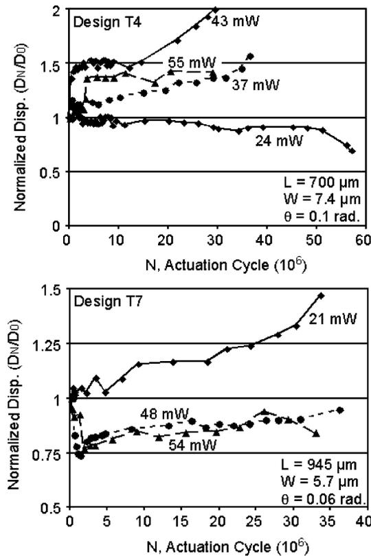
Fig. 8. Displacement variation for polysilicon single-beam designs T4 and T7 at various actuation power levels.
