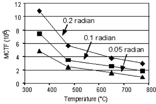
Fig. 10. Mean Cycles to Failure (MCTF) observed for  $p^{++}$  Si actuator designs 1–3.
