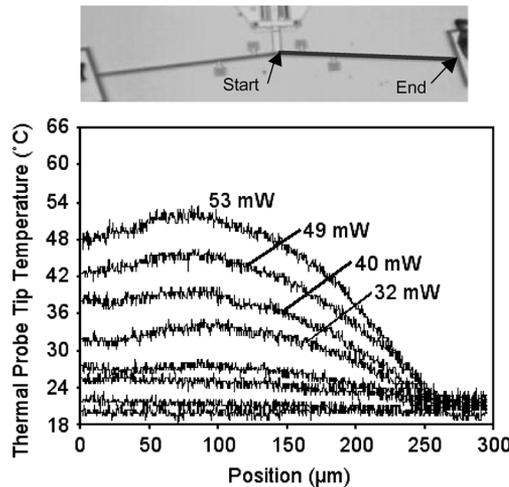
Fig. 5. Temperature profile of a bent-beam obtained using a scanning thermal probe method. The plotted temperature rise is proportional to, but lower than, the actual increase.
