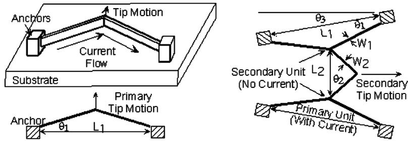
Fig. 1. Structure and operation of a single bent beam actuator (left) and cascaded design (right).
