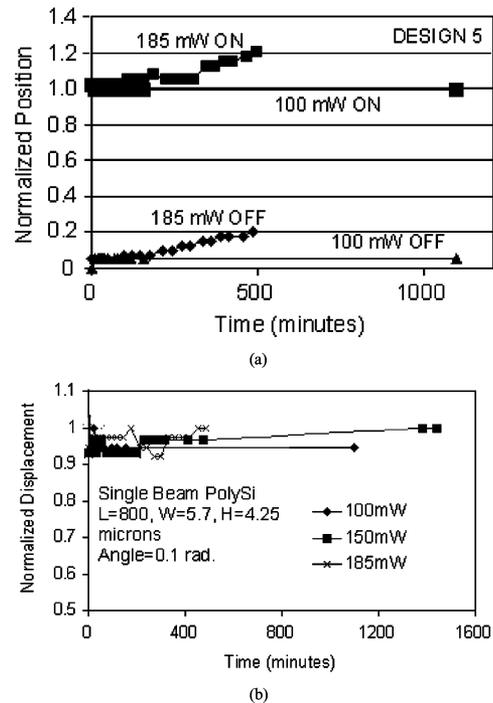
Fig. 6. Measurements of design 5 devices. (a) The power-on and power-off positions normalized to the initial activated position. The plot shows increase by equal amounts over extended periods at high input power. (b) The net displacement, which is the separation between power-on and power-off positions, remains relatively stable.
