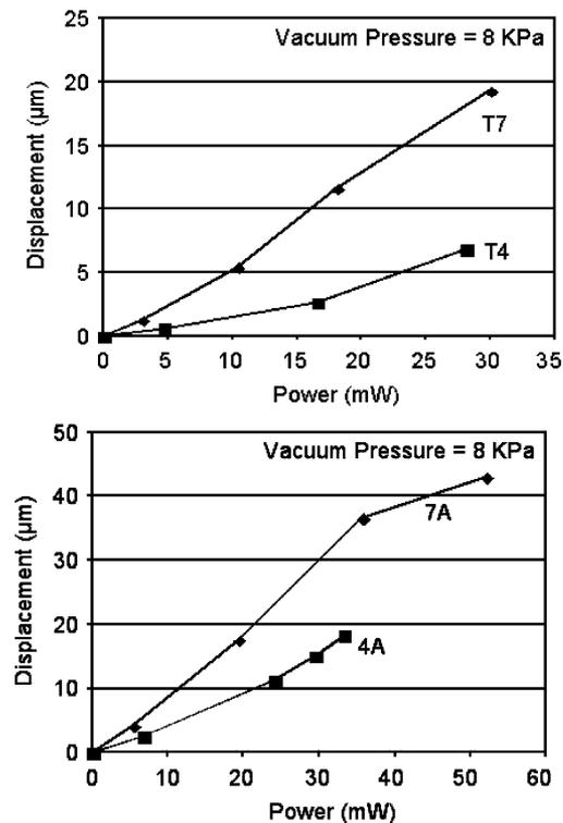
Fig. 3. Measured polysilicon actuator displacement (a-upper) for single and (b-lower) cascaded beam actuator. These results were obtained using dc actuation.
