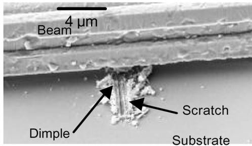
Fig. 12. Dimples that were deliberately formed on the lower surface of the beams to reduce stiction after the sacrificial release during fabrication can rub against the substrate, causing friction.
