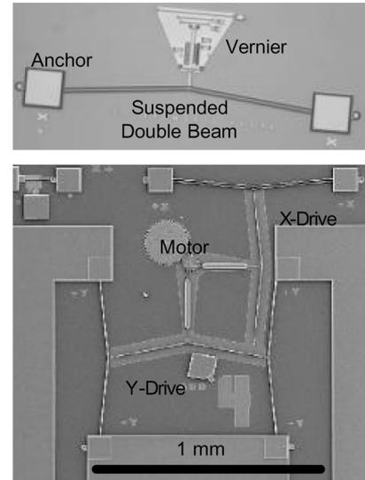
Fig. 2. Fabricated polysilicon microactuators: (a-upper) Optical micrograph of a T4 device, (b-lower) SEM image of a rotary micromotor that used such actuators.
