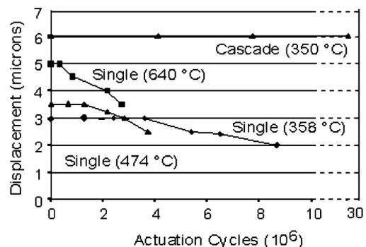
Fig. 7. Pulse activation results for SCS actuators comparing the single beam design 2 at three different temperatures, to the cascaded design 4.
