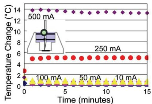
**Fig. 6** Temperature change at the septum entry point over time for recharging currents from  $10\text{--}500 \text{ mA}$ . The circle in the inset denotes the temperature sampling location. The test was conducted in an air ambient environment with a baseline temperature of  $22.4^\circ\text{C}$
