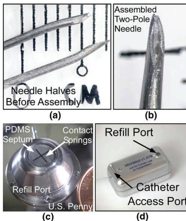
**Fig. 4** (a) Photographs of 26 gauge coated needle halves before and (b) after assembly taken on a white ruler. (c) A photograph of an assembled refill port in which the top contact spring of the septum is clearly visible. The port is pictured here with a US Penny. (d) An implantable drug delivery device with the refill port and a similar catheter access port
