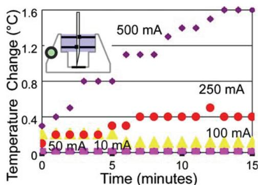
**Fig. 7** The temperature change of the exterior of the port housing for battery charging currents ranging from 10–500 mA. The temperature increase has resolution of 0.1°C and was conducted in ambient air with a temperature of 22.4°C. The circle in the inset denotes the temperature sampling location
