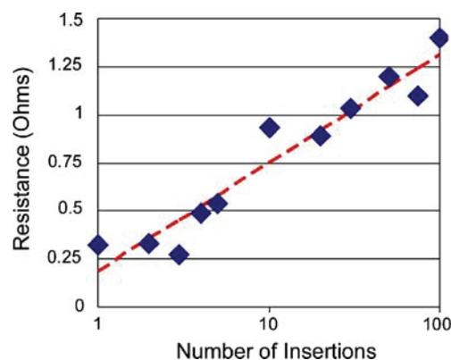
**Fig. 9** The resistance of the needle and spring contact resistance across many insertions with a logarithmic fit. The resistance varies from 0.27–1.4  $\Omega$  over 100 punctures. The logarithmic nature of the resistance indicates that the principal changes to the connection occur early in the life cycle of the refill port
