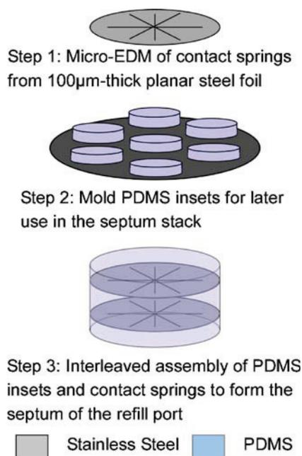
**Fig. 3** The septum is fabricated from biologically compatible materials. Contact springs of various heights to contact with the openings in the needle coating to allow power transfer
