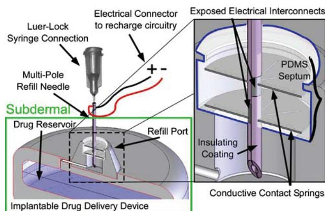
**Fig. 1** The system view: A two-pole needle is inserted into the refill port of a drug delivery device. Inset: A close view of the two needle halves making electrical contact with springs inside the septum
