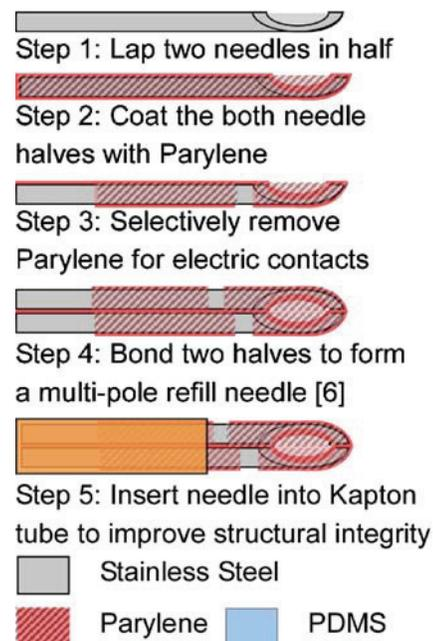
**Fig. 2** The needle is fabricated from biologically compatible materials. The fabrication process creates open conduction paths or “windows” that are self-aligning once inserted into the port
