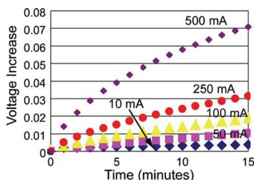
**Fig. 8** The voltage increase of a NiMH 1.2 V AA battery as it is being recharged across a refill port with various charging currents. Typical starting voltages range from 1.1 V to 1.4 V. Charging profiles match expected values, and demonstrate power transmission with acceptable heating rates for a smart needle and port to be used in implantable drug delivery devices
