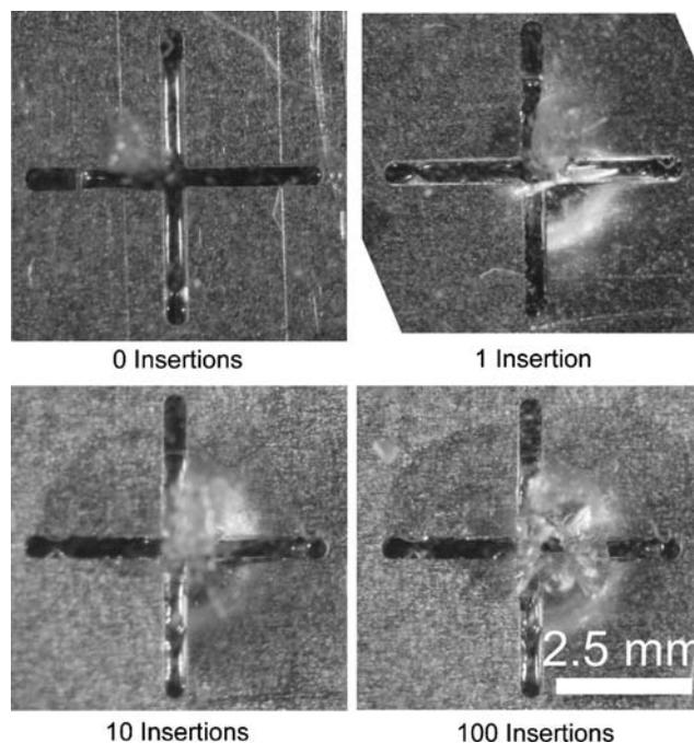
**Fig. 10** Photographs of the needle septum after a set number of punctures taken under a microscope. The photographs reveal that almost all of the spring deformation occurs during the first needle insertion, and subsequent punctures cause minimal mechanical alteration to the port
