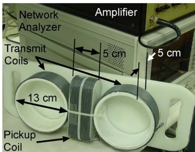
**Fig. 4** Extracorporeal configuration used in the *in situ* testing as fabricated, with important dimensions. Coaxial cable connections to the pickup coil and transmit coils are on the back of the mount
