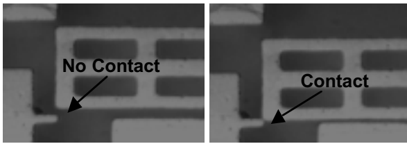
Fig. 7: Optical images showing a proof mass before (left) and after (right) static self-test actuation.
