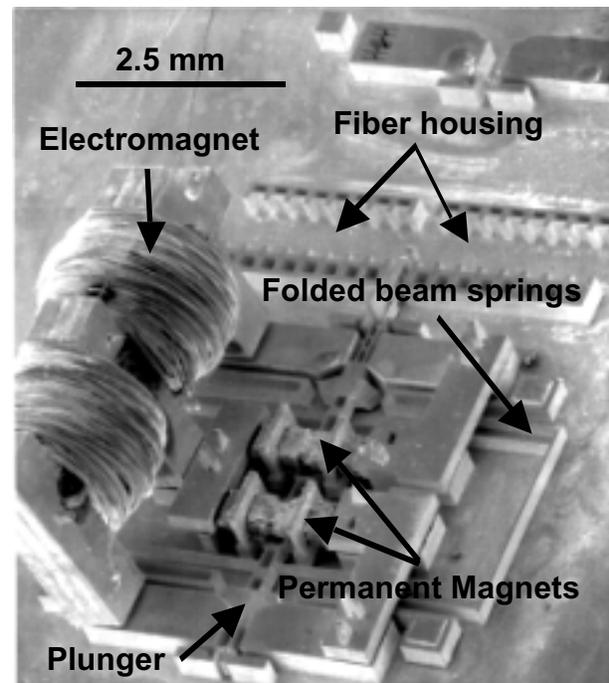
**Fig. 1:** SEM of the bi-directional linear actuator. The length of the permanent magnets is 1.5 mm.
