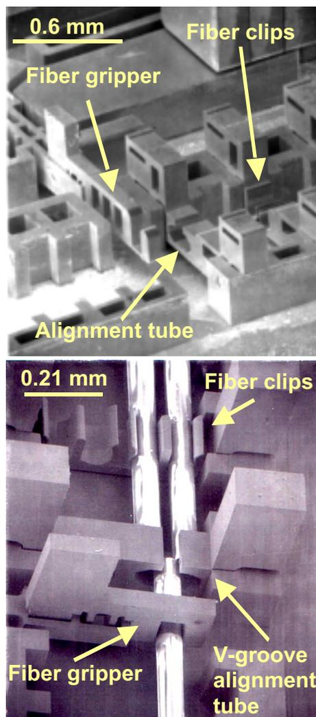
Fig. 5: (a-upper) Alignment tubes and fiber clips without optical fibers; (b-lower) Similar mechanism with optical fibers included.
