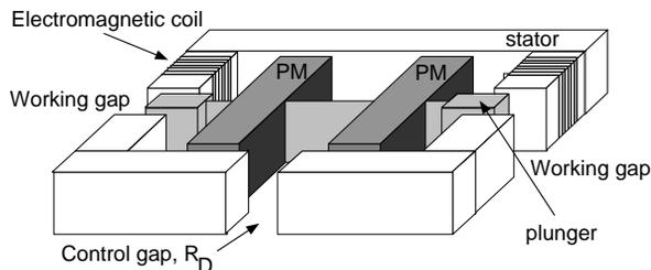
Fig. 2: Concept drawing of the bi-directional magnetic actuator. All material in the core and the plunger are high permeability.
