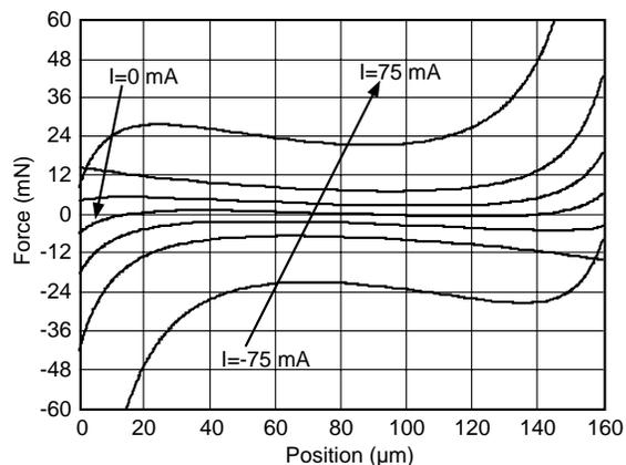
Fig. 4: Theoretical force profiles for the actuator with a 60 degree wedge. The zero current curve shows the latching force when the coils are de-energized.
