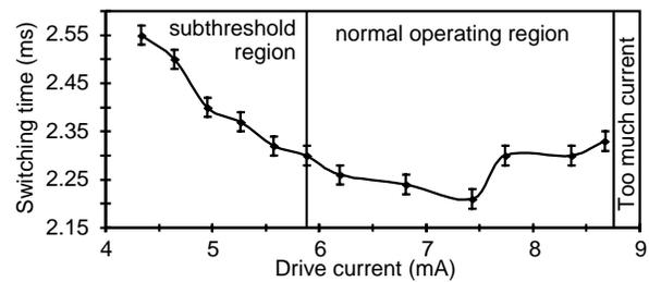
Fig. 6: Measured switching time of actuator.
