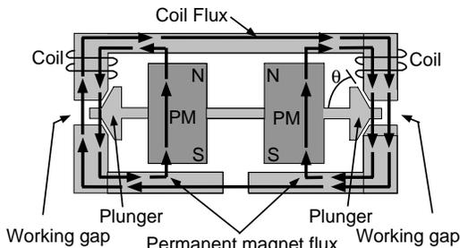
Fig. 3: Flux paths of the magnetic actuator showing the various important components.
