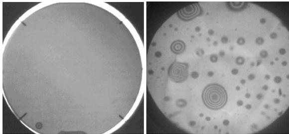
Fig. 7: IR images of a wafer pair before (left) and after (right) anneal for 5 min. at  $1000^\circ\text{C}$ . Voids are created from residual water when very high ramp rates are used with either RF or microwave heating.
