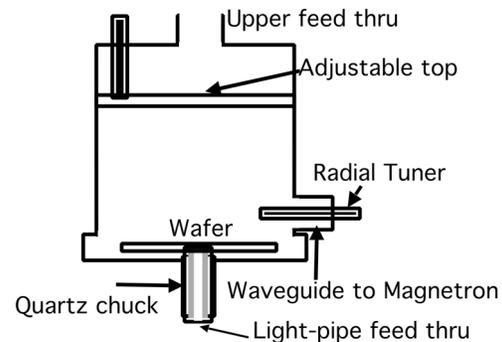
**Fig. 1:** Schematic of the cylindrical resonant cavity used for microwave heating. The cavity is azimuthally symmetric.
