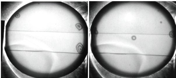
Fig. 6: IR images of EMIH bonded wafers heated for 5 minutes at  $1000^\circ\text{C}$ . Left: microwave. Right: RF
