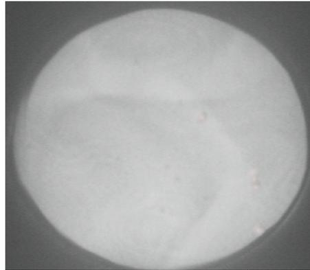
Fig. 8: IR image of wafers with  $2500 \text{ \AA}$  oxides bonded by a 4 min. microwave EMIH anneal at  $1000^\circ\text{C}$
