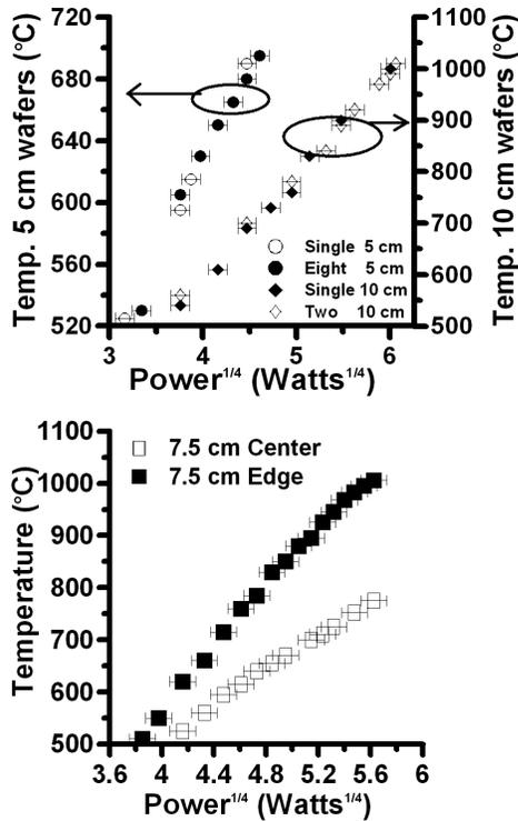
Fig. 5: (a-upper) Steady-state temperature for single and paired 50 mm and 100 mm wafers. The 50 mm wafers were in TM011 mode, while the 100 mm wafers were in TM111 mode. (b-lower) Center and edge temperatures of a 75 mm wafer in the RF system.
