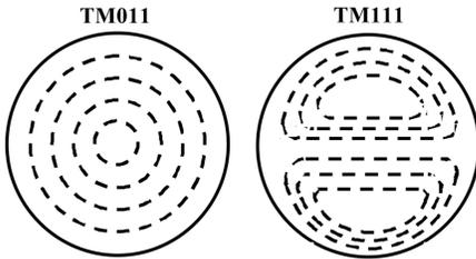
Fig. 2: Magnetic field patterns in the microwave cavity for TM011 and TM111 modes in the plane of the wafer.
