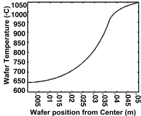
Fig. 4: Semi-analytical solution to the temperature distribution on a 100 mm diameter wafer during RF heating with a spiral coil antenna.
