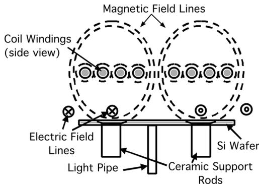
Fig. 3: Schematic of RF system showing induced magnetic and electric field lines.
