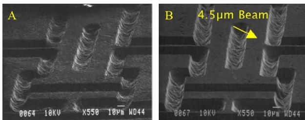
Figure 6. A: Workpiece for uncoated case with much more surface roughness than B: coated case. 4.5 $\mu$ m wide, 1mm long beams.
