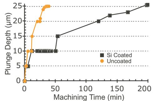
Figure 2. A measurement of plunge depth vs. machining time shows that the uncoated case reached 25 $\mu\text{m}$  quickly while the coated case stalled. This is because the uncoated tool wears down rapidly, and provides a machining depth that is much smaller than the plunge depth.
