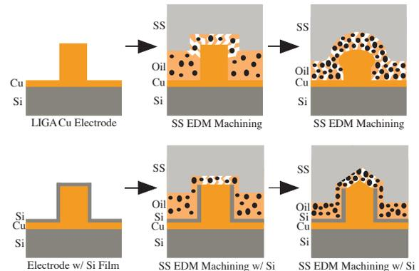
Figure 1. Comparison of machining progression for uncoated tool (top) and passivation coated tool (bottom). Rounded workpiece edges and melted tool for uncoated case and selective machining for coated case.
