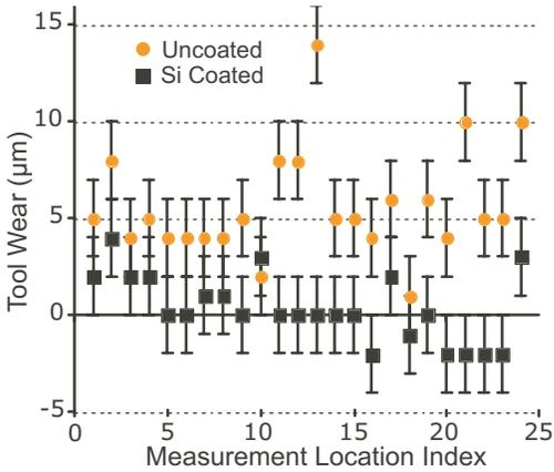
Figure 5. Si coated tool wear was less than uncoated tool
