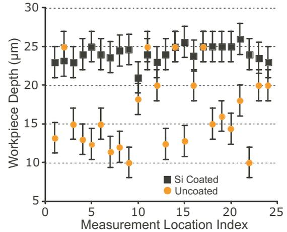
Figure 3. Uncoated workpiece did not machine the full  $25 \mu\text{m}$  in most areas and also varied excessively across the pattern compared to coated case.
