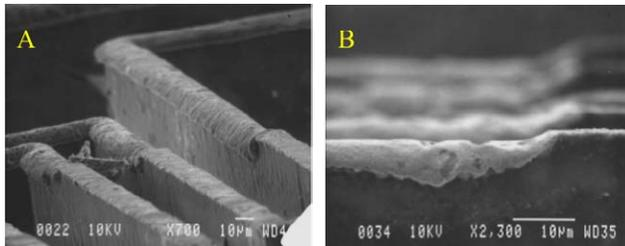
Figure 7. A: Uncoated tool transition from unmachined (bottom) to mushroom shape (top). B: Si coating wears down as copper wears slowly. Right side is unmachined, left side shows exposed copper top.
