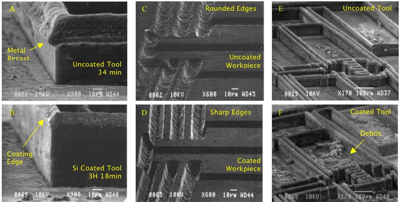
Figure 4. A: Uncoated tool recasts into a mushroom shape after machining. B: Silicon coated tool has negligible wear. C: Uncoated workpiece with feature rounding, edge rounding, and rough surfaces. D: Coated workpiece with sharp features, sharp edges especially on corners, better surface finish, and much deeper machining. E: Used uncoated tool has mushroom shape across all features. F: Used coated tool with low wear and large debris on surface.
