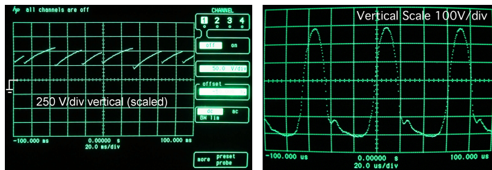
Fig. 4: (a: left): Oscilloscope trace of circuit output while creating pulsed arcs with a 3 V battery; (b: right): Measured waveform at the test point in the absence of a discharge, with a 1.5 V battery.
