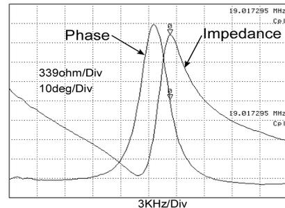
**Fig. 8:** Screen print of Agilent 4395 impedance analyzer, showing the measured impedance of a quartz disk in the array with a typical piezoelectric resonance peak in air at atmospheric pressure.
