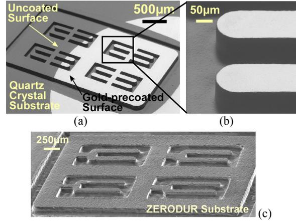
**Fig. 5:** ESEM images of: (a) an array of H-shaped patterns transferred onto a quartz crystal substrate by the process; (b) close-up view of the structure, showing the vertical sidewall formed in the batch mode  $\mu$ USM. Cutting depth:  $\approx 105$   $\mu$ m. Note that the machining did not remove the gold layer pre-coated on quartz. (c) SEM image of an array of tuning fork patterns transferred onto a ZERODUR substrate. Cutting depth:  $\approx 100$   $\mu$ m.
