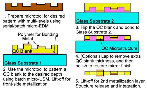
Fig. 1: Schematic diagram of the proposed process flow for quartz crystal microstructure with multi-levels.
