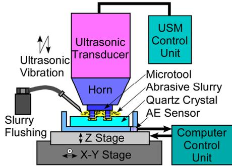
Fig. 2: Schematic diagram of the  $\mu$ USM setup for batch-mode pattern transfer onto quartz crystals. Acoustic emission (AE) sensor is used for dynamic process monitoring and control.
