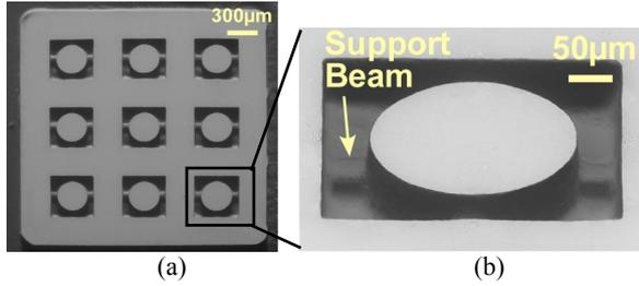
**Fig. 4:** Photos of: (a) PZT disc array batch fabricated by SEDUS process using batch  $\mu$ USM to transfer a pattern defined by serial  $\mu$ EDM. (b) Released PZT disc. Diameter: 200  $\mu$ m. Thickness: 50  $\mu$ m.
