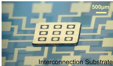
**Fig. 7:** Photo of the disk array mounted on a substrate with metal interconnections using silver epoxy, showing the concept of on-chip integration with other MEMS and circuit devices. The top common electrode is to be wire bonded.
