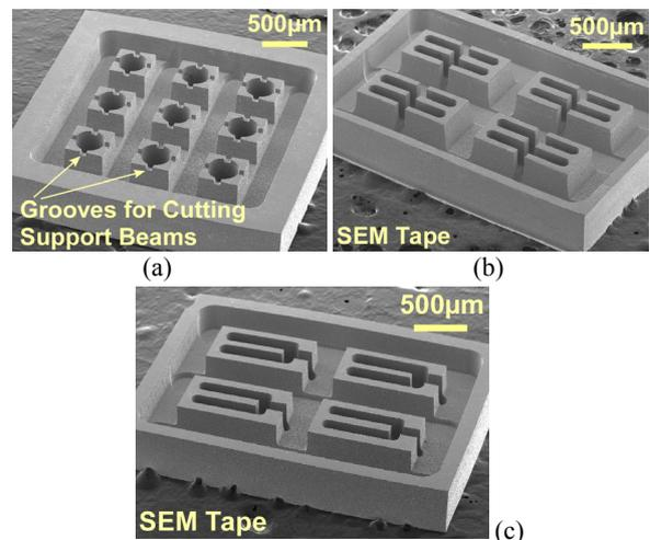
Fig. 3: SEM images of microtools made by serial mode  $\mu$ EDM for: (a)  $3 \times 3$  array of disks; each supported by four  $50 \mu\text{m}$ -wide beams formed by the grooves; (b)  $2 \times 2$  array of H-shaped structures; (c)  $2 \times 2$  array of tuning fork resonators.
