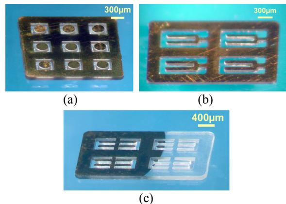
**Fig. 6:** Photos of the released quartz crystal structures. (a) Disk array ( $\approx 85$   $\mu$ m thick); (b) H-shaped structure array ( $\approx 100$   $\mu$ m thick); (c) tuning fork array ( $\approx 75$   $\mu$ m thick). Note the scratches in (a) & (b) are only on the metal layers.
