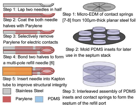
Figure 4: The needle and septum are fabricated from biologically compatible materials. The fabrication process aligns the conductive needle windows to the springs so they make contact upon insertion.
