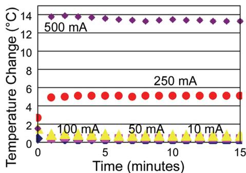
Figure 10: The temperature change of the exterior of the port housing for battery charging currents ranging from 10-500 mA. The temperature increase has resolution of 0.1°C and was conducted in ambient air with a temperature of 22.4 °C.
