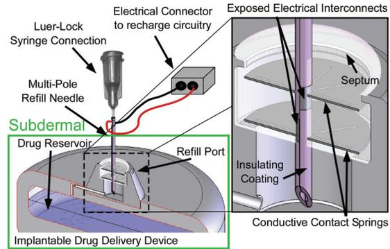
Figure 1: The system view: A two-pole needle is inserted into the refill port of a drug delivery device. Inset: A close view of the two needle halves making electrical contact with springs inside the septum.
