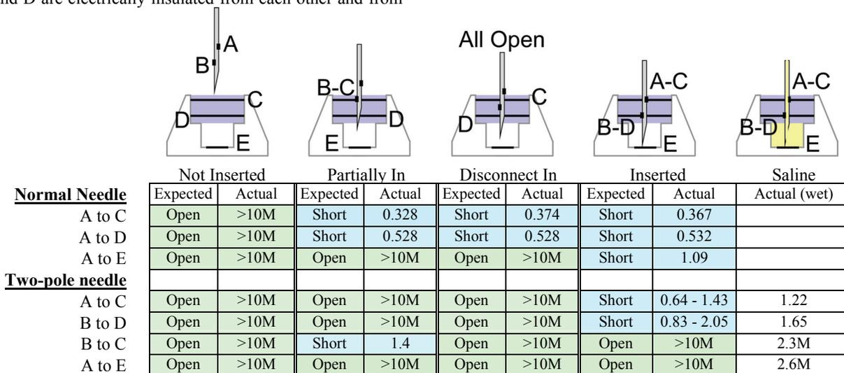
Figure 8: Stages of insertion with resistances color coded to expected states for normal and split needles both dry and completely filled with saline after insertion. (\*All resistances are in Ω)
