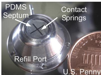
Figure 7: A photograph of an assembled refill port in which the top contact spring of the septum is clearly visible. The port is pictured here with a US Penny.
