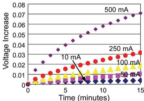
Figure 11: The voltage increase of a NiMH 1.2V AA battery as it is being recharged across a refill port with various charging currents. Charging profiles match expected values, and demonstrate power transmission with acceptable heating rates for a smart needle and port to be used in IDDDs.
