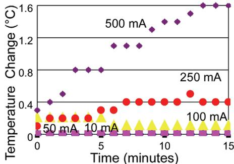
Figure 9: Temperature change at the septum entry point over time for recharging currents from 10-500 mA. The test was conducted in an air ambient environment with a baseline temperature of 22.4 °C.
