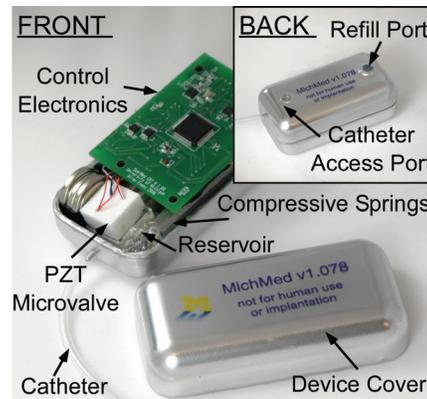
Figure 2: A photo of the front of an assembled microvalve-regulated drug delivery device with the back side refill port shown inset [8].
