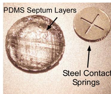
Figure 6:  $\mu\text{EDM}$  springs and PDMS septum layers.
