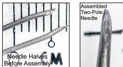
Figure 5: Photographs of 26 gauge coated needle halves before and after assembly taken on a white ruler.
