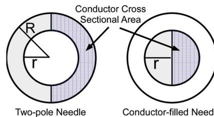
Figure 3: Two possible needle configurations. Either the needle is split (left) or it is filled with a conductor (right).
