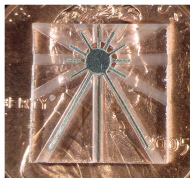
Figure 3: Pressure sensor with electrodes spaced 50 \mu\text{m} apart and 125 \mu\text{m} in thickness on a U.S. penny.
