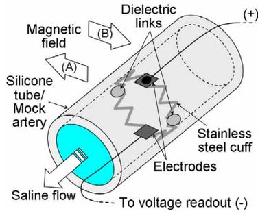
**Fig. 9:** A close-up of the device in the set-up with different orientations of magnetic field.
