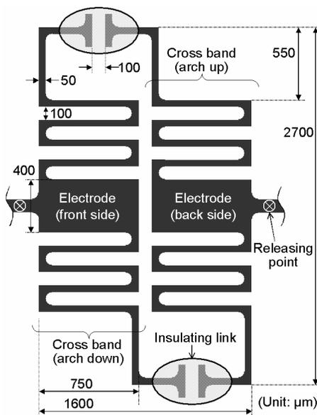
Fig. 2: A layout of the planar cuff structure.
