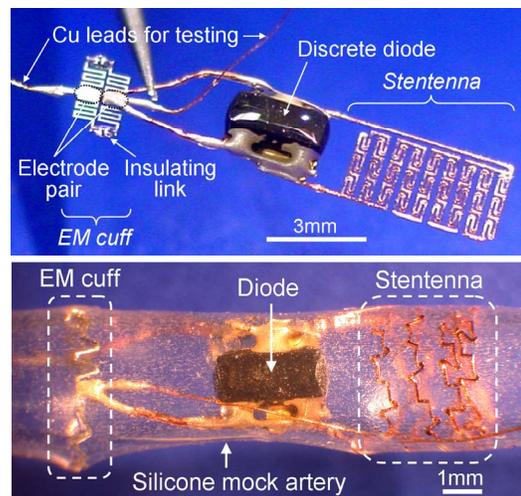
**Fig. 12:** (a: upper) The planar state of a fabricated hybrid device, and (b: lower) the device deployed inside a mock artery tube.
