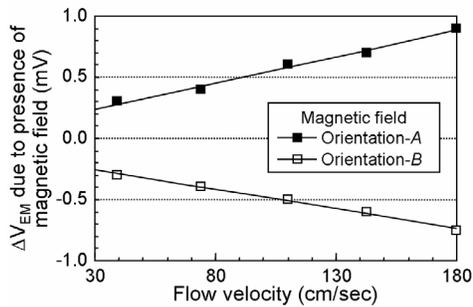
**Fig. 10:** Measurement result showing linear dependence on flow velocity and symmetric responses with opposing magnetic fields.
