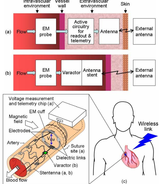
Fig. 1. System architectures for (a) active monitoring, and (b) passive implementation. (c) Illustration of sample placements of devices in scheme (a) and (b).
