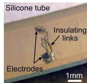
Fig. 7: The cuff remains attached to the inner walls of the tube by pressure after the balloon is deflated and removed. (The lead wires have been removed.)
