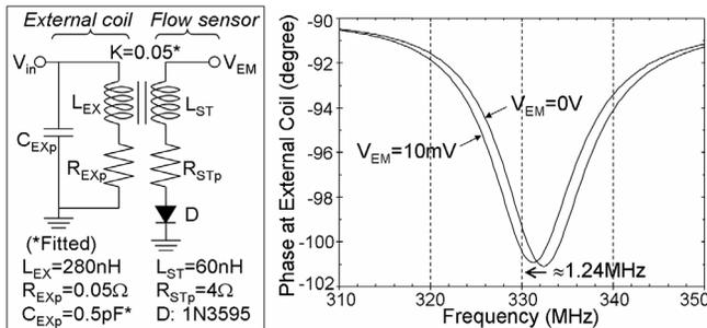
Fig. 15: (a: left) SPICE model of the wireless set-up, and (b: right) simulation result showing a shift of L-C tank resonance due to  $\Delta V_{EM}$ .
