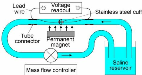
**Fig. 8:** A set-up for flow measurement.
