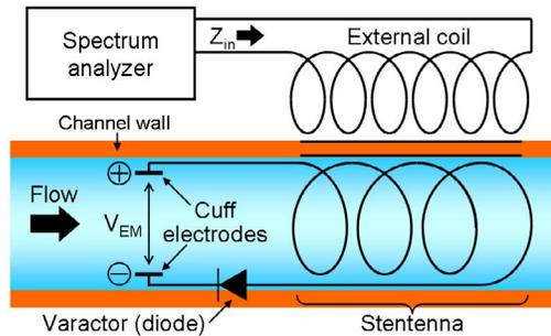
**Fig. 11:** The concept of the intraluminal passive device and its telemetry setup.
