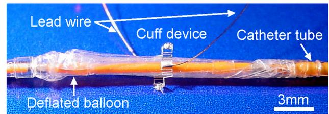
Fig. 5: A planar cuff structure mounted on a standard catheter balloon in the deflated state.
