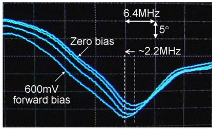
Fig. 13: Measured shift in phase dip of external with emulated  $V_{EM}$  varied by 200mV per step.
