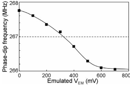
Fig. 14: Measured frequency shift with the emulated  $V_{EM}$ .
