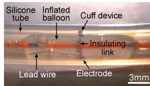
Fig. 6: The planar cuff plastically expanded to a ring shape inside a silicone tube by inflation of the balloon.
