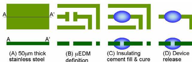
Fig. 3: Fabrication process flow [11].
