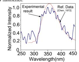
Fig. 8: The net output from the tryptophan sample, obtained by subtracting the curve of Fig. 7 from that of Fig. 6. The reference emission curve of tryptophan [6] has been superimposed.
