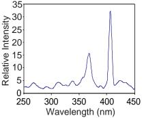
Fig. 7: Spectrum measured with a DI water control sample in a manner analogous to Fig. 6, shows the absence of the broad peak between 325 nm and 425 nm.
