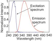
Fig. 1: Typical excitation and emission spectra of tryptophan show that the UV source must operate over 250-290 nm wavelengths, whereas the fluorescence peaks over 330-390 nm [5,6].
