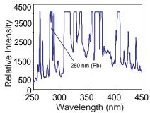
Fig. 3: Measured spectrum from lead nitrate with concentration of 5g/10ml water (saturated solution), showing substantial emission intensity in the 250-290 nm wavelengths.
