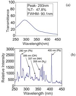
Fig. 4: (a) Transmission curve of the filter separating the UV source from the tryptophan sample. (b) Measured spectrum of the filtered emission, showing increased prominence of 250-290 nm wavelengths as compared to the unfiltered emission in Fig. 3.
