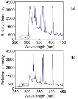
Fig. 5: (a) Light transmitted through tryptophan shows that the peaks near 280 nm have been absorbed; (b) These wavelengths are transmitted through the control sample of water.
