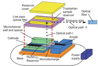
Fig. 2: An exploded schematic of the device showing various components. The tryptophan sample reservoir can be replaced by a micro-total analysis chip.
