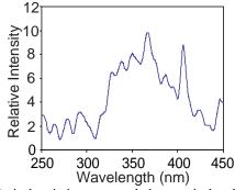
Fig. 6: Optical emission measured along optical path II (as shown in Fig. 2) indicating the existence of the direct fluorescence of tryptophan by the broad peak between 325 nm and 425 nm.
