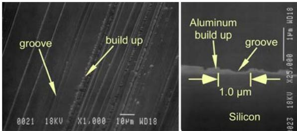
Fig. 2: SEM image of Al film abraded by alumina grit tool.
