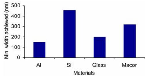
Fig. 5: Minimum width achieved for each substrate by using alumina grit tool.
