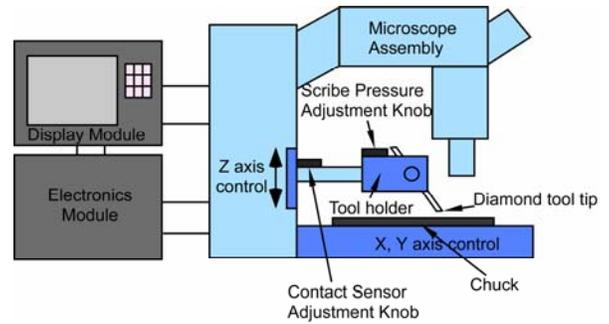
Fig. 1: A schematic of the abrasion tool.
