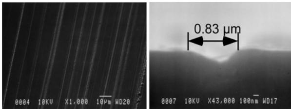
Fig. 3: SEM image of single crystal Si abraded by alumina grit tool.
