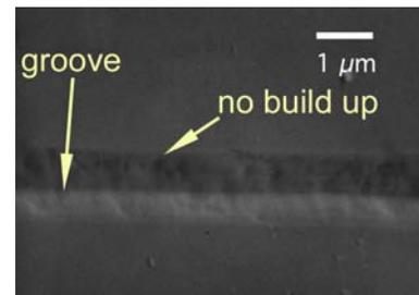
Fig. 7: SEM image of top view of single crystal Si abraded with diamond tool head.
