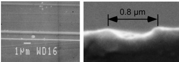
Fig. 4: A #7740 Pyrex™ glass sample abraded by alumina grit tool.
