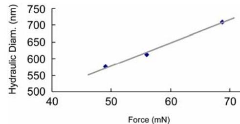
Fig. 8: Hydraulic diameter of Si grooves achieved by varying applied force using diamond tool.
