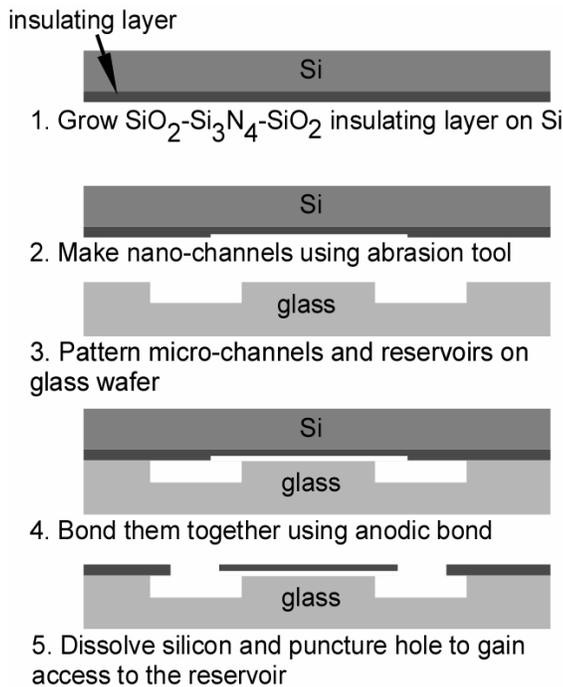
**Fig. 9:** Process flow diagram for applying the abrasion method for non-lithographic fabrication of channels of sub-micron hydraulic diameter combined with conventionally micro-machined features.
