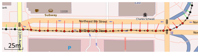
(a) Red samples match to the lower road in ground truth, which is a one-way road in reverse direction.
