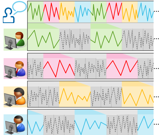
Figure 1. TimeWarp forwards different “warped” versions of the audio to each worker. Workers hear a slowed down version of the content they are supposed to caption, while they hear the rest sped up. This increases the quality of workers’ output by asking them to complete an easier task without losing context. The start of each slowed segment is aligned with the original audio, allowing the crowd to collectively caption in real time.
