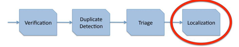
Fault localization (FL): the task of identifying the files that could be changed to address the defect.
