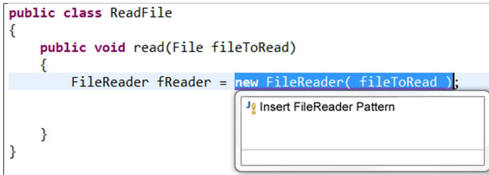
Figure 7.1: Mock-up of an API-usage auto-completion tool. In this case the user has declared and initialized a FileReader object. The tool responds by suggesting to complete the full pattern associated with this API.
