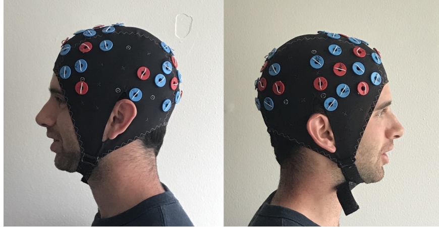
Figure 4.2: fNIRS Cap Photograph: fNIRS cap used in our experiments. Red circles are light transmitters while blue circles are light receivers. fNIRS is only able to observe brain activation on channels between nearby transmitters and receivers.
