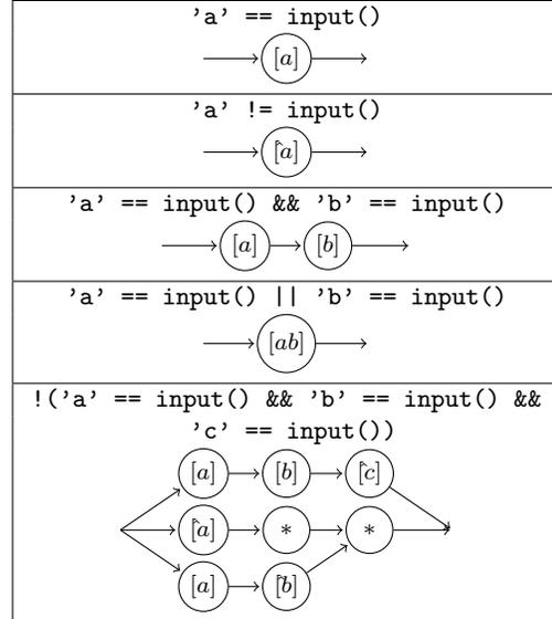
Figure 7: Example transformations of RAPID expressions into automata
