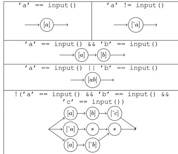
Fig. 8. Example transformations of RAPID expressions into automata
