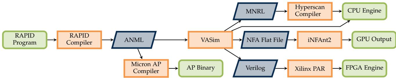
Fig. 11. Supported pipelines for executing RAPID programs. RAPID programs can be executed on CPUs (using VASim or Hyperscan), GPUs (using iNFAnt2), FPGAs, and Micron’s D480 AP. Rounded green boxes indicate the input and output of the pipeline. Orange rectangles are software tools used to generate intermediate and output files. Blue parallelograms are intermediate files generated by our pipeline.
