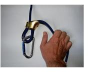
Mountain climbing and carabiners are associated with this. In this common activity, tension and friction help ensure safety. These devices act as friction brakes, and allow the climber to easily vary the amount of friction on the rope by altering the rope's position. In one position, the rope runs freely through the device. In another position, it can be held ("locked off") without the rope sliding through the device because of the friction on the rope.
