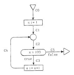
Let us note [a, b] where  $a \le b$  the predicate  $a, \le x \le b$ . The system of equations corresponding to the example is :
