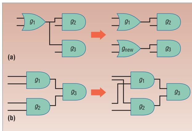
**Figure 5. Case studies. (a) Cell  $g_1$  has insufficient driving strength; SafeResynth uses a new cell,  $g_{new}$ , to drive a fraction of  $g_1$ 's fanouts. (b) SymWire reduces coupling between parallel long wires by using symmetries to change their connections. This also changes metal layers and can alleviate the antenna effect.**
