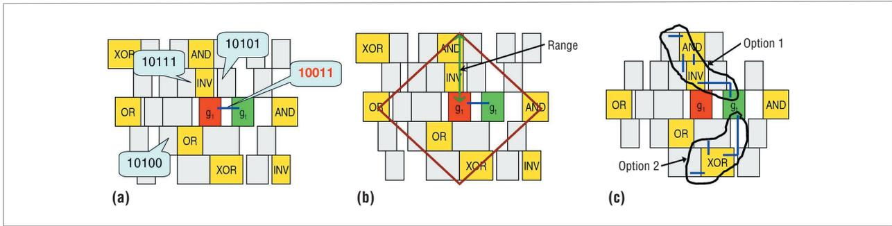
**Figure 4. Functional error repair in an integrated circuit. (a)** PAFER diagnoses that the wire driven by  $g_1$  is erroneous and provides a corrected partial truth table using other cells as inputs. **(b)** PARSyn uses spare cells to perform Boolean manipulation of the signals, restricting its search to cells within a predicted range. **(c)** The algorithm generates various resynthesis netlists with different combinations of inputs and spare cells.
