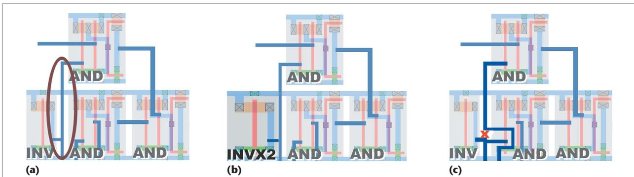
**Figure 1.** Postsilicon error repair example. (a) Original buggy layout with a weak driver (INV). (b) A traditional resynthesis technique finds a simple fix that sizes up the driving gate, but it requires expensive remanufacturing of the silicon die to change the transistors. (c) Our physically aware techniques find a more complex solution using symmetry-based rewiring, but it can be implemented with a metal fix and has a smaller physical impact.
