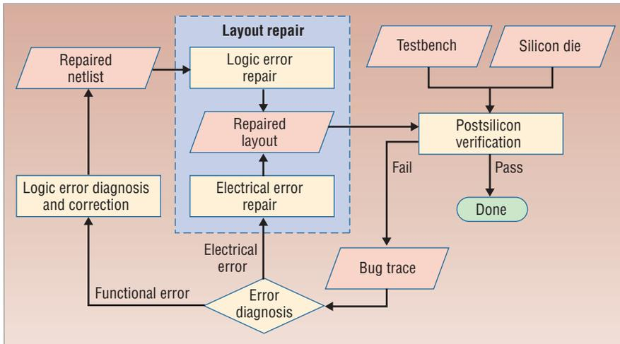
**Figure 2. Current postsilicon debugging methodology.** To validate a silicon die, engineers apply numerous test vectors to the die and then check their output responses. If the responses are correct for all the applied test vectors, the die passes validation. If not, the test vectors that expose the design errors become the bug trace, which engineers use to diagnose and correct the errors.
