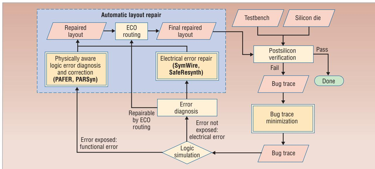
**Figure 3. FogClear postsilicon debugging methodology.** We first use bug trace minimization to reduce a trace's complexity. We then simulate the trace with a logic simulator to identify the error as functional or electrical. Next, we determine whether the error can be repaired by ECO routing tools or electrical error repair techniques. Finally, we route the repaired layout via ECO to produce the final layout, which we use to fix the silicon die for further verification.
