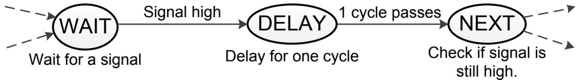
**Figure 5.2 Portion of an FSM for a protocol checker.** The delay state is needed only for checking strict timing, which can at times be relaxed.
