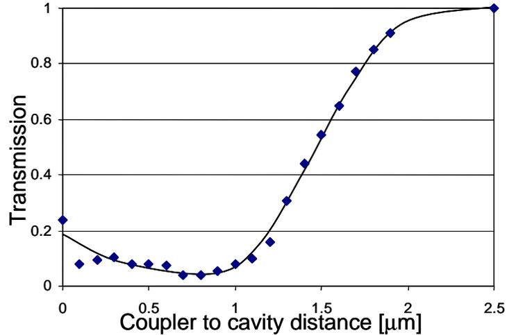
Fig. 4. Experimental measurement of the bent-coupler transmission Vs. coupling distance (squares); the line is a guide for the eye. Cavity external diameter is  $32\ \mu\text{m}$  with minor diameter of  $6\ \mu\text{m}$ , coupler outer diameter is  $37\ \mu\text{m}$  with minor diameter  $3.5\ \mu\text{m}$ . Optical quality factor is 22 million and wavelength is  $1542.4\ \text{nm}$ .
