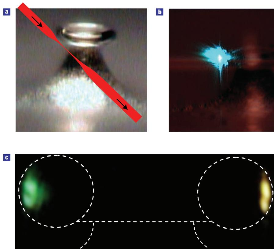
**Figure 1** Third harmonic generation from a microtoroid. **a**, Photograph of the silica microtoroid structure used by Carmon and Vahala<sup>2</sup> along with the tapered fibre shown schematically (red). **b**, Blue emission from infrared pumping of the microtoroid, where the microtoroid is still dimly visible. **c**, Green and yellow emission generated with two different-wavelength counter-rotating pump lasers. (Images reproduced from ref. 2).
