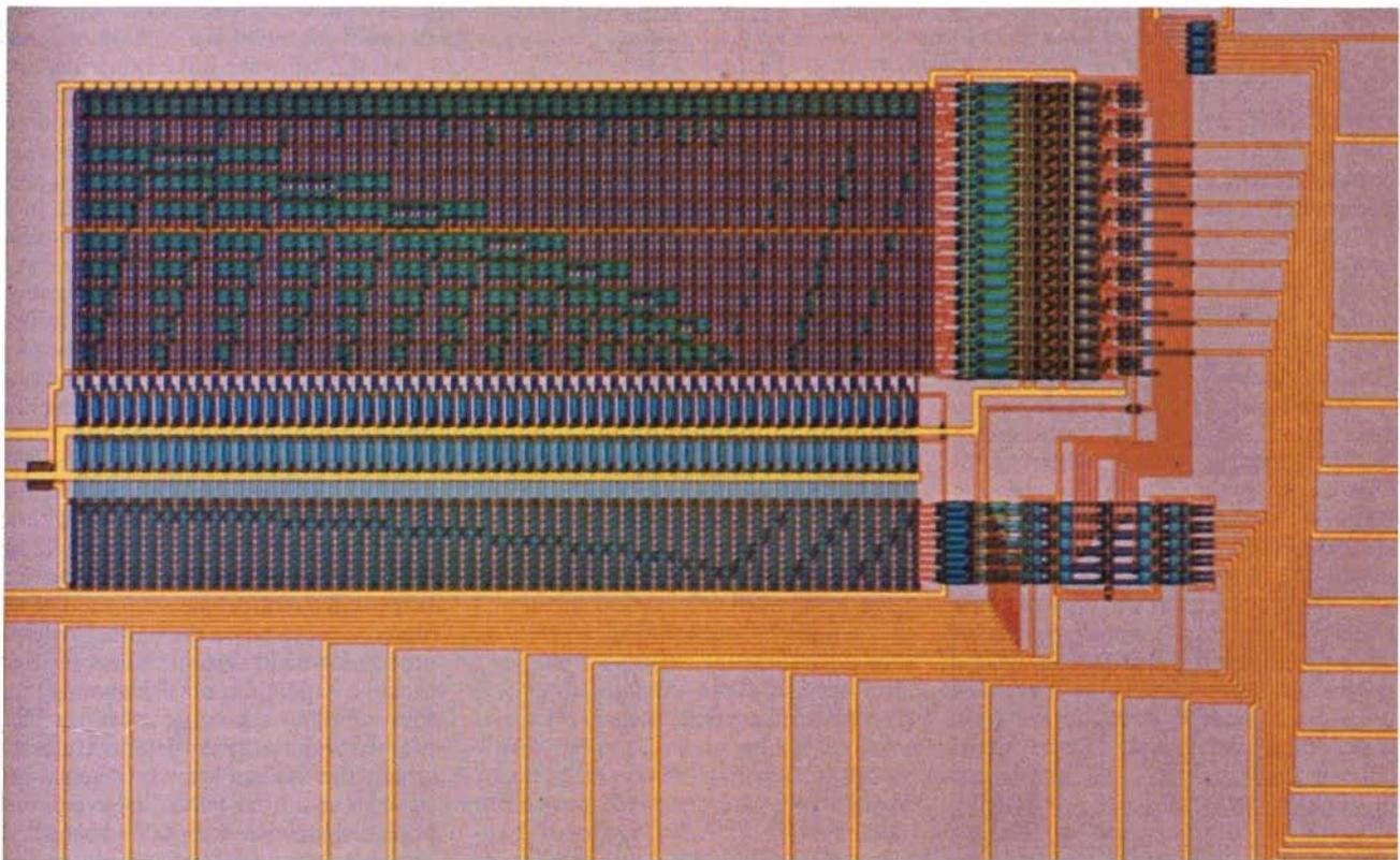
CONVENTIONAL COMPUTING DEVICES, the abacus and **the** logic chip, both dissipate energy when they are operated. The “**log-**ic gates” central to the design of a chip expend energy because they discard information. A chip consumes energy for a less fundamen-**tal** reason as well: it employs circuits **that** draw power even when they merely hold information and do not process it. The abacus is
