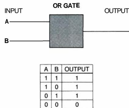
**CONVENTIONAL LOGIC GATES** dissipate energy because they discard information. For example, if the output of an *and* gate is 0, there is no way to deduce what the input was.
