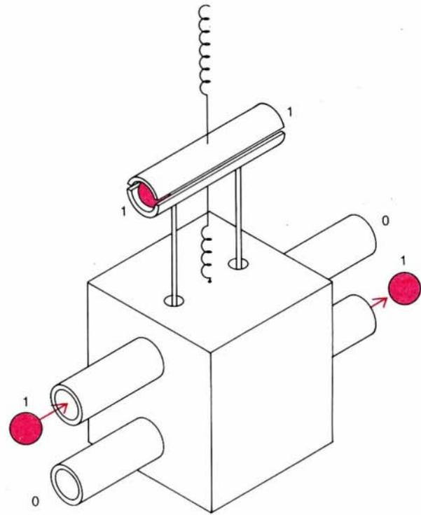
**IDEALIZED PHYSICAL REALIZATION** of a Fredkin gate substitutes pipes for wires and the presence or absence of a ball for a 1 or 0. A narrow, split segment of pipe represents the control channel. When a ball passes through it, the pipe spreads apart, operating a switching mechanism; the mechanism in turn switches any input ball from line A to line B and vice versa. A pair of springs keeps the
