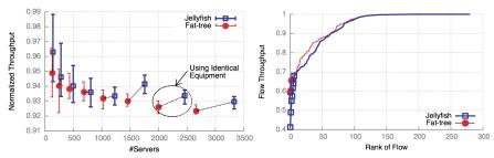
1) Jellyfish has better throughput than Fat-tree, even with sub-optimal routing
