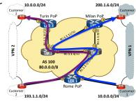
Datagram sent to customer's network using tunneling (i.e., an MPLS label-switched path)
