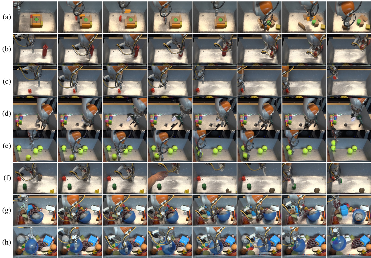
Figure 4. Eight grasps from the QT-Opt policy, illustrating some of the strategies discovered by our method: pregrasp manipulation (a, b), grasp readjustment (c, d), grasping dynamic objects and recovery from perturbations (e, f), and grasping in clutter (g, h).
