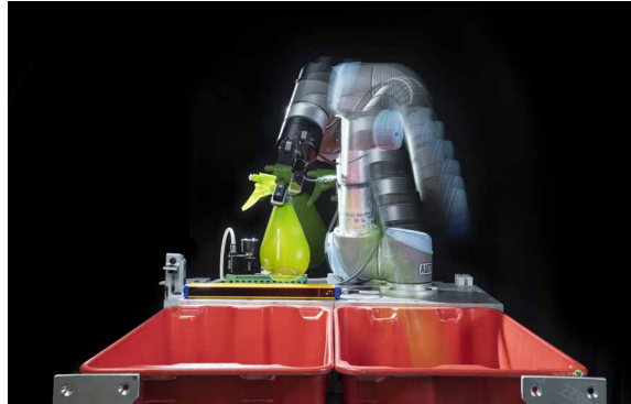
Fig. 1. Grasp-optimized motion planning in action. The proposed motion planner computes a time- and jerk-optimized motion for pick-and-place operations, using a combination of deep learning and optimization. Time optimization makes the motions fast (sub-second). Jerk (change in acceleration) optimization avoids overshooting and reduces wear over long term repeated operation. For a given pair of start and end robot configurations, deep learning rapidly computes an approximation of the optimal motion that can violate motion constraints (e.g., collides with a bin, exceeds joint limits). The motion planner then feeds the approximation to an optimization process to minimize jerk and fix up the constraint violations. By using the deep-learning-based approximation, the computation time speeds up by 300x.
